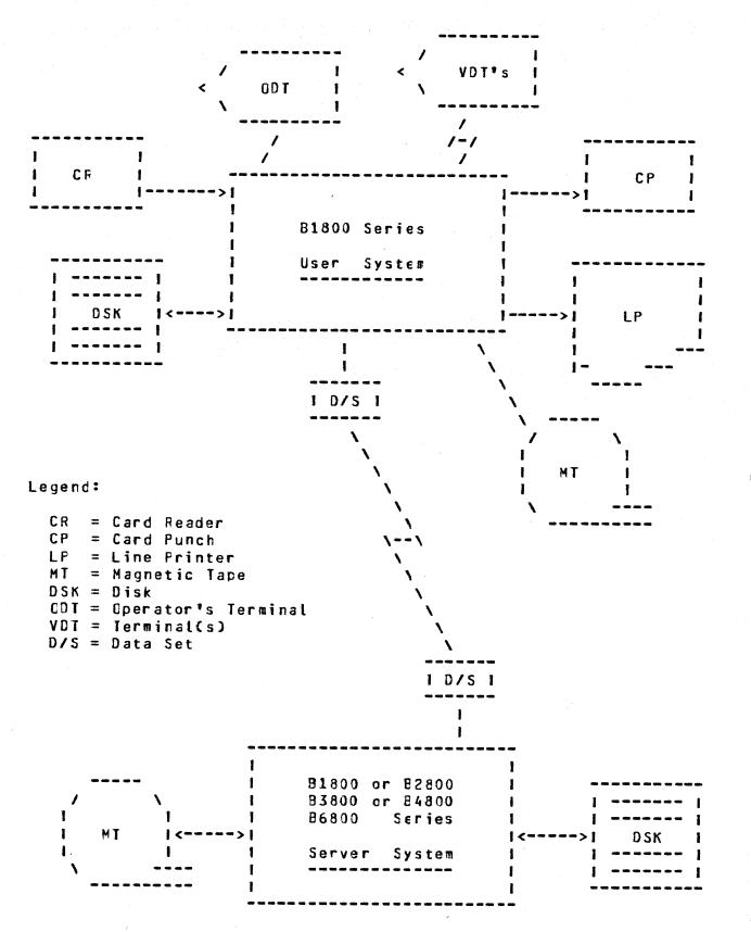
Figure 3-4: User System - Server System Schematic
