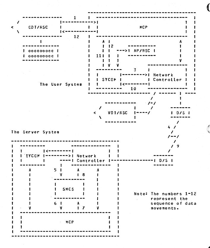
Figure 4-2: RSC Input/Output Message Flow
