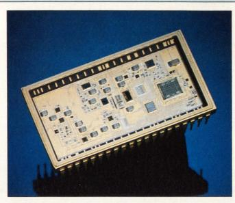
Hybrid A-D converters such as Comlinear's CLC935 still have a performance advantage over monolithic parts. This 12-bit, 15-Msample/s part maintains a 77-dB spurious-free dynamic range at 7.22 MHz. Signal-tonoise ratio is 66 dB out to Nyquist rates (7.5 MHz).
