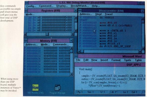
You can view registers, data memory and disassembled program memory simultaneously.
