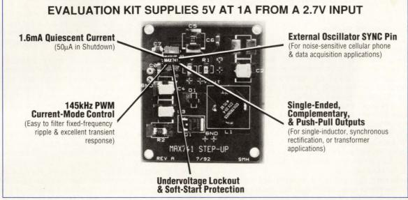
A complete pre-assembled surface-mount evaluation kit demonstrates disk-drive and palmtop applications: stepping up to 5V at 1A from a 2.7V input—order the MAX741UEVKIT-SO kit. For 5V, 1.5A output step-down applications, order the MAX741DEVKIT-SO kit. \$30.00 each.
