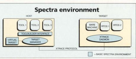
Ready Systems' Spectra environment supplies a common interface for development and debugging tools on the host system. Tools communicate with the real or a virtual target via the same interface. The shaded blocks identify the basic Spectra components.
