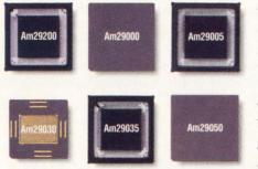
The 29K Family includes parts for every conceivable applicationfrom the brand new low cost, easy-to-use Am29200<sup>TM</sup> to the top-of-theline Am29050<sup>TM</sup> with on-chip floating point coprocessor. they provide everything you need to speed up the design process, every step of the way. From evaluation, to system and hardware design, software development, hardware and software integration, system debug—all the way to production.
