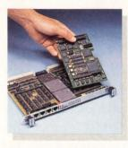
Over a dozen smart, powerful I/O modules fit Synergy's '020, '030, '040 and Dual '040 SBC's
