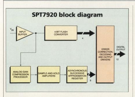
The SPT7920 from Signal Processing Technologies is the industry's first 12-bit, highspeed, monolithic A-D converter. Available with 10-Msample/s and 30-Msample/s speeds, the chip offers a signal-to-noise ratio of 67 dB (typical). To achieve this level of performance, SPT used a non-traditional, proprietary architecture.
