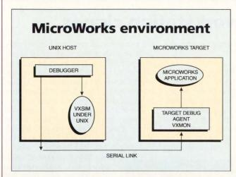
software runs as a UNIX process using the Sunos lightweight process mechanism to manage context switching. "You're writing C source and debugging with VxGDB, whether you do it on the host or target," Barbagallo says. "When the hardware comes in, you just recompile and download."
