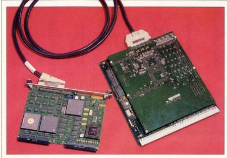
CCT is offering the first Futurebus+-to-VMEbus bridge, comprising two boards: a 12-SU Futurebus+ card and a 6U VME card. The boards provide the essential link between the two buses, offering Futurebus+ systems much needed I/O. The bridge allows multicage distributed processing, shared memory structures between cages and Futurebus+ access to any existing VMEbus I/O devices. With the bridge, the Futurebus+ system can become a master on the VMEbus system, and vice versa.
