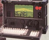
Conduction Cooled Housing with optional Liquid Cooling
