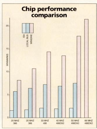
The most common benchmark among chip set vendors is the Winmark suite. These numbers, from Chips and Technologies, show over 20 million Winmarks of performance for a 486DX2based system with a Wingine accelerator.
