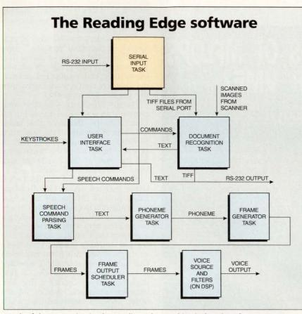
Much of the processing in The Reading Edge machine is done in software. Images are received from the scanner, converted to text and broken down into phonemes. These phonemes are divided into discrete time segments called frames. The frames are sent to the DSP, where they modify filters that control the speaker output.
