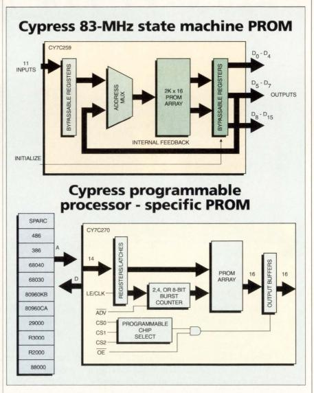
By integrating registers, feedback and counters with fast PROM cores, Cypress has created two high-speed specialty PROMS. One (A), for complex state machines with relatively few inputs (11 max), can run at 83 MHz. The other (B), for instruction storage, can service virtually any of the fastest RISC and CISC processors.
