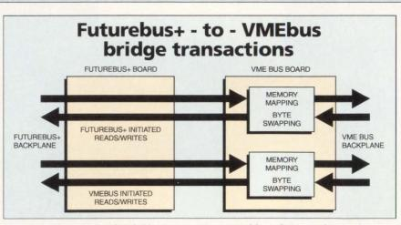
CCT's Futurebus+-to-VMEbus bridge maps a memory address from one bus to the other. Inherent in the memory mapping scheme is the ability to swap bytes around when different processor types are used. The bridge also permits multiple crates to be tied together in a star or daisy-chain configuration.
