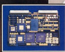
The Fire Control Processor for the M1A2 Abrams Main Battle Tank: one example of Vista Controls' fully mil-qualified RISC-based board-level systems solutions for fire control and gun stabilization. Being manufactured today.
