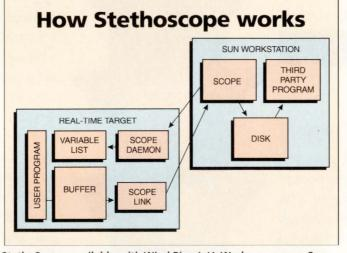
StethoScope, available with Wind River's VxWorks, runs on a Sun workstation and interacts remotely with the target via the real-time signal manager module, called ScopeDaemon. The target program places data in a buffer that is transferred to StethoScope via the ScopeLink cod, which is designed to have a minimal impact on target performance. A third-party program, such as Matlab from Mathworks, can be used to analyze and process numeric data.
