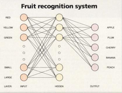
In this simple neural network, a layer of inputs lists the various characteristics of fruit. When the network gets a stimulus from one or more of these inputs, it responds with an output. If the network guesses incorrectly, it adjusts the correlation of the internal connections or synaptic weights until it gets a correct answer.
