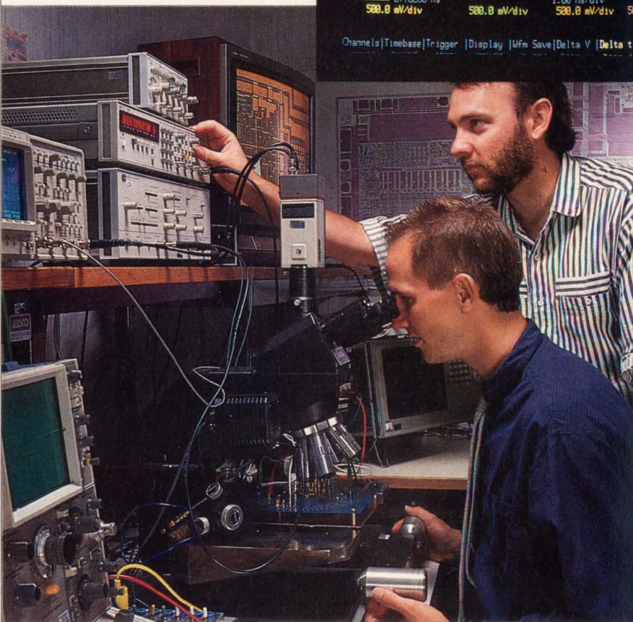
Gazelle designers Gary Gouldsberry, standing, and Bob Burd examine the phase-shifting characteristics of Gazelle's PLL-based clock distribution chip (inset). It locks TTL-compatible clock outputs to a master signal, but with phase shifts programmable in 2-ns increments. The company claims the accuracy of the phase shift is typically ±100 ps.
