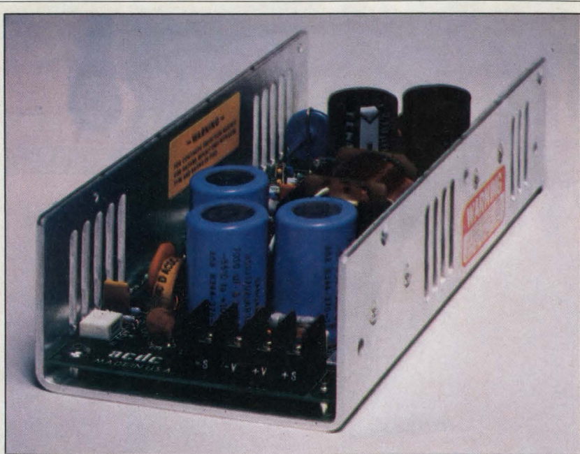
Higher frequency reduces the size of this 100-kHz, 100-W, single-output switcher from ACDC Electronics. This 4- x 8- x 2.2-in. (10.16- x 20.32- x 5.59-cm) supply is one of the first on the market to use power MOSFETs.
