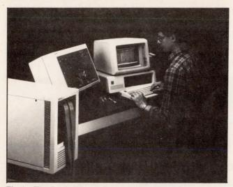
Fig 1 The Logic Master Series of functional testers puts integrated stimulation, acquisition, and realtime comparison into the hands of the IC designer already using the IBM PC.
