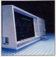
Liberal use of built-in intelligence sets the HP 54100 oscilloscope apart as a thoroughly modern instrument for engineers studying gigahertz-range waveforms. This unit features a  $5\frac{1}{2}$ - x 7-in. electromagnetic screen (4- x 6-in. useraccessible), 500 x 256 pixel resolution, and screen generated graticules.
