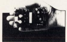
Triple output power supplies of 30 W are key to the 3030 series. For example, the 3030-1 board measures 3- x 5- x 1.8-in. (76.2- x 127- x 45.7-mm), and weighs 0.5 lb. These compact units operate with low output noise and feature 4000 Vac I/O isolation, tight line/load regulation, and user-selectable input voltage ranges of 90 to 130 Vac and 180 to 250 Vac. Cost is \$69. **Power General**, 152 Will Dr, PO Box 189, Canton, MA 02021 **Circle 353**
