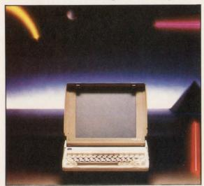
Smaller than a briefcase and weighing only 9.1 lb, Data General's One personal computer is operationally compatible with the IBM PC. It runs the MS-DOS and CP/M-86 operating systems using a 4-MHz 80C88 CMOS microprocessor. The unit's LCD shows a full 25 lines of 80 chars on a screen. Double 3<sup>1</sup>/<sub>2</sub>-in. disk drives located at the side of the keyboard/chassis, provide up to 737 Kbytes of memory. To top it off, a basic package with one disk drive costs only \$2895.
