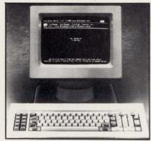
The PC Shadow offers the appearance of 25-line PC operation and a similar keyboard. It supports IBM graphics characters, and screen attributes such as reverse video, highlighting, blinking, and low intensity. The PC Shadow also supports an auxiliary printer port with a transparent data path that supports X-ON/X-OFF protocols. Users can select the Televideo 925 emulation mode s an option. Price is \$895. Software Link, Inc, 8601 Dunwoody Pl, Atlanta, GA 30338. Circle 368
