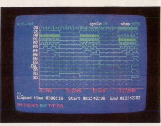
Fig 3 During the logic simulation phase, the engineer can view outputs from PC-LOGS as graphical waveforms. The simulation can be started and stopped at any time, with up to 16 output states probed at once.
