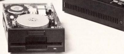
FD-35 Series 3.5-Inch Micro Floppy Disk Drives Capacities from 250 KB – 1 MB. Interface Compatible with 5½ " Floppy Disk Drives. Power Saver Version: 1.72 watts Read/Write, 2.9 watts Seek, 27 milliwatts Waiting.
