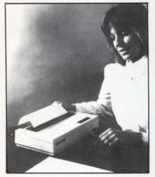
Measuring 13 x 7.5 x 2.8 in.  $(33 \times 19 \times 7.1 \text{ cm})$  and weighing 6.6 lb (2.9 kg), the GLP printer is intended as a portable computer companion. It features IBM PC compatibility and PC block graphics, as well as enlarged, condensed, emphasized, and double-strike print modes. The GLP is available with a Centronics parallel interface, or with both RS-232 and Centronics interfaces combined in one unit. Price is \$299. **Centronics**, 1 Wall St, Hudson, NH 03051. **Circle 381**
