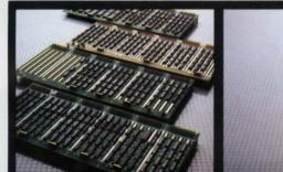
Over 450 ICs from these four boards were squeezed onto two VLSI graphics co-processor chips – in only six months.
