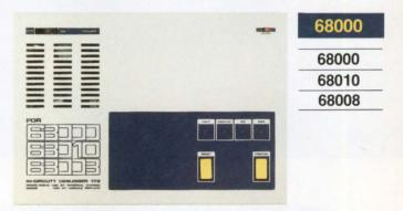
Emulates 68000, 68008 and 68010 in one unit to 10 MHz. Features; 128K of emulation memory – expandable to 256K, 4K deep x 48 bits wide realtime trace buffer, 30 different debugger commands.
