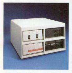
For large configurations, choose the DSX80000 foundation system with eight Multibus slots, 10, 20, 40 or 80Mb of Winchester storage plus an 8" IBM compatible floppy.
