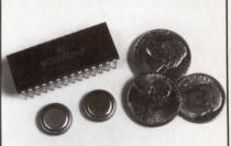
The MC68HC04P2/P3 8-bit computers on a single chip contain CPU, onchip clock, 1or 2-Kbyte ROM (plus 72 bytes for lookup tables), and 32 or 128 bytes of RAM, as well as memory mapped I/O. With software features similar to those of M6800 family members, these devices sport 20 TTL/CMOS-compatible bidirectional I/O lines (eight LED-compatible lines). Volume pricing is approximately \$4. **Motorola Inc, MOS Microprocessor Div**, 3501 Ed Bluestein Blvd, Austin, TX 78721. **Circle 363**
