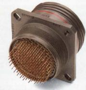
Filtered Military/Aerospace Connectors. Intermateable and intermountable with standard Mil-Spec circulars as well as MIL-C-24308 rectangulars. Amphenol® and Bendix® filtered connectors pass desired low frequency signals while attenuating line conducted EMI/RFI. These connectors are also designed for maximum protection from radiated EMI/RFI. Available in a broad range of filtering characteristics, shell sizes, styles and contact termination options.
