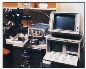
Engineers presently using VLSI design automation tools available on VAX computers can now test chip designs on the Tektronix DAS 9100 logic analysis system. The 91DVV VLSI verification software package from Tektronix creates a close relationship between the VAX host and logic analyzer. This combination implements chip testing more easily and at much lower cost than production testers.
