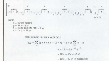
Fig 6 The overhead time of a major cycle is composed of a number of variables: interframe spacing (IFS) time, frame overhead time (f), and a linear delay which varies with the station number. The overhead defined here includes all time intervals outside the information field shown in Fig 5.
