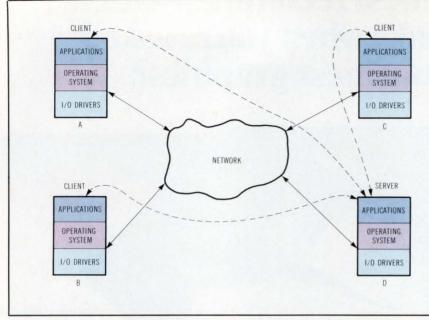
Fig 3 In a typical network there are three clients using one server. Clients cannot communicate directly with other clients, nor can they directly share their resources. Typically, network patches are "inserted" at the junction of the operating system and the 1/0 drivers. This means that whatever data is coming over the net at this level will be strongly flavored by the resident operating system.
