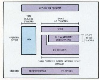
Fig 2 A typical VRTX-based realtime operating system can have four modules that take care of a realtime tasking services interface, the STDIO I/O services interface, the PC-DOS media interface, and the Small Computer System Interface (SCSI) device interface. Other modules are under development. diskettes. The PC-DOS media is, in fact, quite compatible with FMX.
