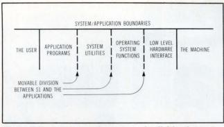
Fig 1 With the S1 operating system, the division between the operating system and application programs is arbitrary. Modules implementing system functions can be linked into applications, and both utilities and applications can be included in the developer-tailored system.
