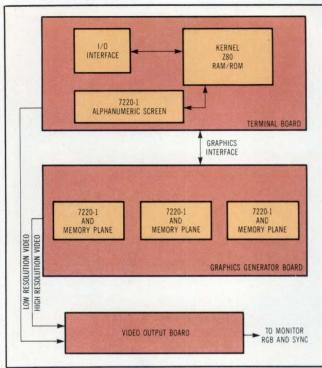
Fig 3 A block diagram of the system shows the principal components—terminal board, graphics generator board, and video output board. The terminal board controls the system sending display commands to the graphics generator, and color map commands to the video output board.
