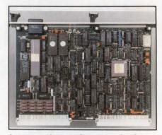
interrupts the MPU for protocol software timing. Physical specs include a double Eurocard form factor, operating temperatures of 5 to 50 °C, and power requirements of 4.4 A at 5 V, and 0.6 A at 12 V.
