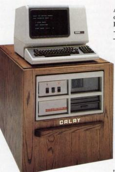
your existing CAD environment the Calay RPR-300 Router and feed it the data from your <u>REDAC</u> or <u>APPLICON</u>. After a short time of the fully automatic routing process, you get the complete data of a routed PC board, which is <u>fed back</u> to your original CAD system for output documentation purposes.
