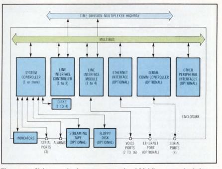
The DSC-2000 Voiceserver implements a conventional Multibus system backplane for conventional data transfers and easy expansion, as well as a 32-channel time division multiplexing highway for voice processing.
