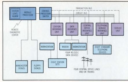
Fig 1 A Telenova 1 module includes a central processor, mass storage devices, and a control processor switch. It has 18 slots for a mix of interface units to connect to central office trunks, station instruments, and a variety of data generating and receiving devices.
