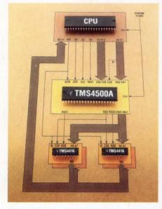
For a cost-effective, low-power memory system that uses minimum board space, combine the TMS4416 or the TMS4164 64K DRAM with the TMS4500A.
