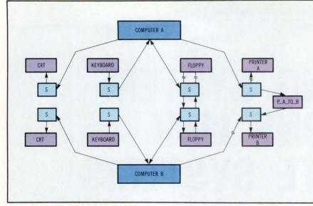
Fig 1 The operating system performs data flow redirection. Control sockets (the boxes marked "S") have been inserted between the peripheral devices and the processor. The CRTs and **KEYBOARDS** are operating normally. Computer A is using computer B's printer. There is a translator program P\_A\_TO\_B that handles mapping control command sequences from printer A to printer B. Computer B is using computer A's floppy drive. In this case, computer A is also using its own floppy drive.
