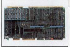
or binary timers/event counters. Its nine levels of vectored interrupt control are expandable off-board to 65. A programmable synchronous/asychronous RS-232-C compatible serial interface offers softwareselectable baud rates.
