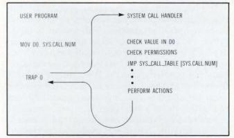
Fig 2 The actual mechanism of system calls is different for its application and system modules. The illustration applies to a Motorola 68000 microprocessor-based s1, but the same principles are used regardless of the microprocessor chosen by the computer designer.
