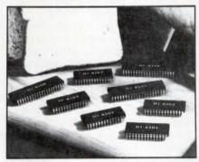
A family of breadboard chips offers a wide variety of analog components that match the operating traits of custom ICs. The HI-8000 series consists of eight CMOS chips that constitute a full array of commonly-used analog components and standard circuits. They simplify the integration of analog circuitry, decreasing semicustom circuit development time. The system supports single- or dual-supply voltages from 1.6 to 18 Vdc. Holt Inc, Integrated Circuits, 8 Chrysler Ave, Irvine, CA 92714. Circle 304
