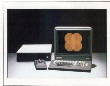
Fig 1 The color graphics terminal incorporates four 7220-1 graphics chips for high speed processing. Design objectives include 1024 x 1024 dot-addressable resolution, smooth pan, and zoom.
