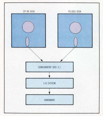
Fig 3 While the Concurrent DOS 3.1 operating system is advanced enough to allow either CP/M- or DOS-based magnetic media, future operating systems will go a step further and support multiple media by permitting system operators to choose a file system at will.
