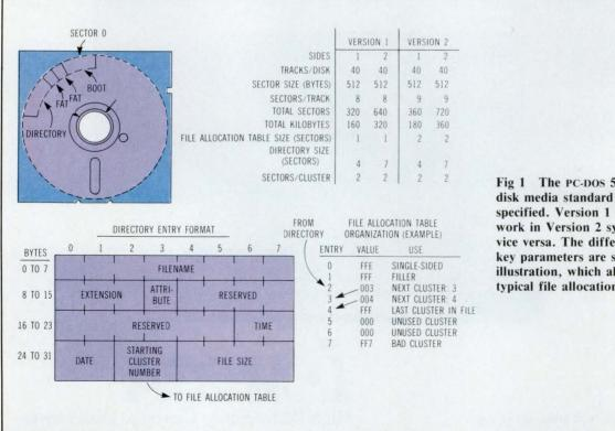
Fig 1 The PC-DOS 5<sup>1</sup>/<sub>4</sub>-in. floppy disk media standard is well specified. Version 1 floppy disks work in Version 2 systems, but not vice versa. The differences in some key parameters are shown in the illustration, which also shows a typical file allocation table.
