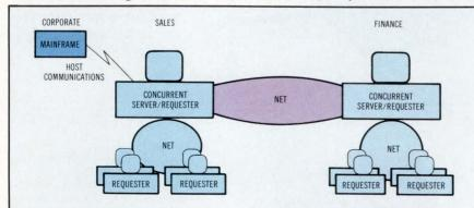
Fig 5 Remote resource identification by the operating system allows it to deal efficiently with networking requests. ID is accomplished by the use of a network specifier in the device name; either a logical mapping or network-ID will do the job for the operating system's service routine.
