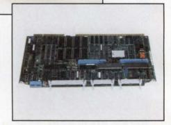
is based on the ANSI proposal for virtual device interface. PROM capabilities of both interpreters provide standard graphics support for the iSBC 186/78, or for an iSBX 275 Multimodule board. The system interfaces to either monochrome or color raster-scan display monitors, has eight universal memory sites for local RAM or ROM store, and provides full RS-343 or RS-170 support.
