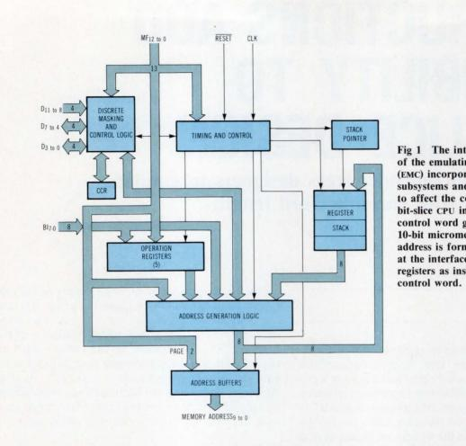
Fig 1 The internal logic structure of the emulating microcontroller (EMC) incorporates most of the subsystems and capabilities required to affect the control section of a bit-slice CPU into one part. A 13-bit control word generates the next 10-bit micromemory address. The address is formulated from inputs at the interface and internal registers as instructed by the control word.
