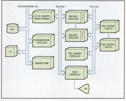
The DS-1 workstation performs pipelining operations beginning in the micromainframe processor and continuing in the Multibus processors. Any of the Multibus processors can read/write pixel data or control information into pixel memory. The video controller converts pixel memory information into RGB intensities.
