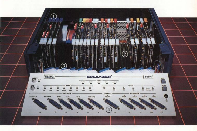
The raw power and flexibility required to tackle your bit-slice, microprogrammed, or other high performance processor-based designs head-on is in the DS370. No other system uses bit-slice architecture. This builtin power emerges in the versatile logic analyzer and integrated writable control store, graphic performance analysis, selective trace, symbolic debug, and 16 triggering levels.
