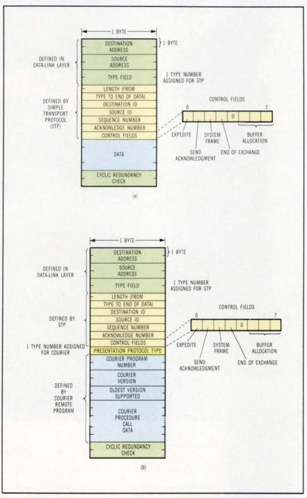
Fig 6 The complete serial backplane frame structure (a) includes the data-link and transport protocol layers adapted from Ethernet. The Courier call (b) also includes a protocol defined by the Courier remote program.
