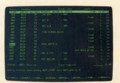
Trace photo of internal data bus is example of how the HP 64264S Emulator shows you more of the 8051 internal operation than ever before.
