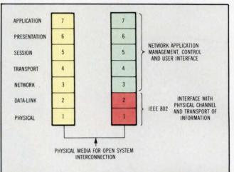
Formalizing standards can reduce confusion among vendors and customers alike. Helping to clarify local area network specification, the IEEE 802 standard is compatible with the lowest two layers of the seven-layer International Standards Organization Open System Interconnection model.
