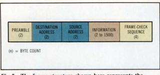
Fig 5 The frame structure shown here represents the protocol by which data is passed between stations on the short-topology LAN. This structure is set by the transport layer when a station is first powered up.
