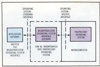
The IEEE's Microprocessor Operating System Interface (MOSI) Task Group 855 is charged with devising a standard interface so that application programs can communicate with diverse operating systems. The interface will translate system calls and functions as shown.
