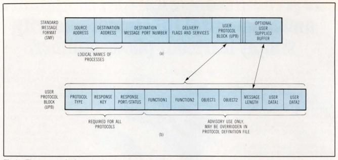
Fig 4 The TNOS standard message format (SMF) in (a) includes the user protocol block (UPB) in (b). Part of the UPB is optional and may be suppressed by the particular protocol in use. Similarly, there is an optional user-supplied buffer in the standard message format.
