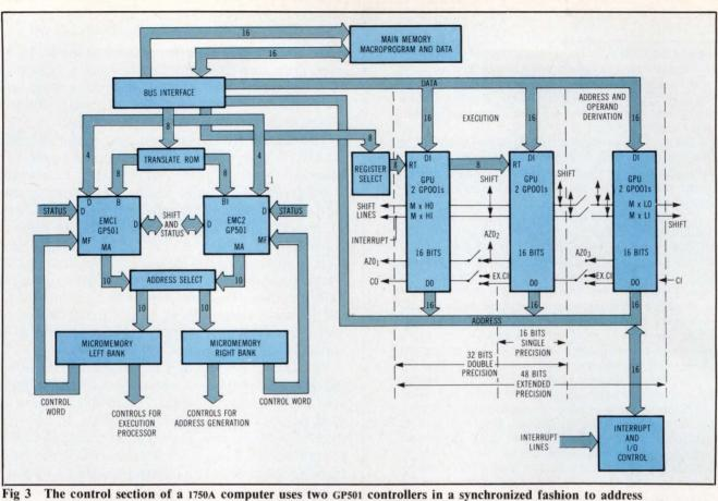
Fig 3 The control section of a 1750A computer uses two GP501 controllers in a synchronized fashion to address micromemory. Concatenated 8-bit ALU slices form the general processing section which comprises an execution part, and an address and operation generation part. Operations can be performed on 16-, 32-, and 48-bit wide data. A few LSI parts tie the whole system together.
