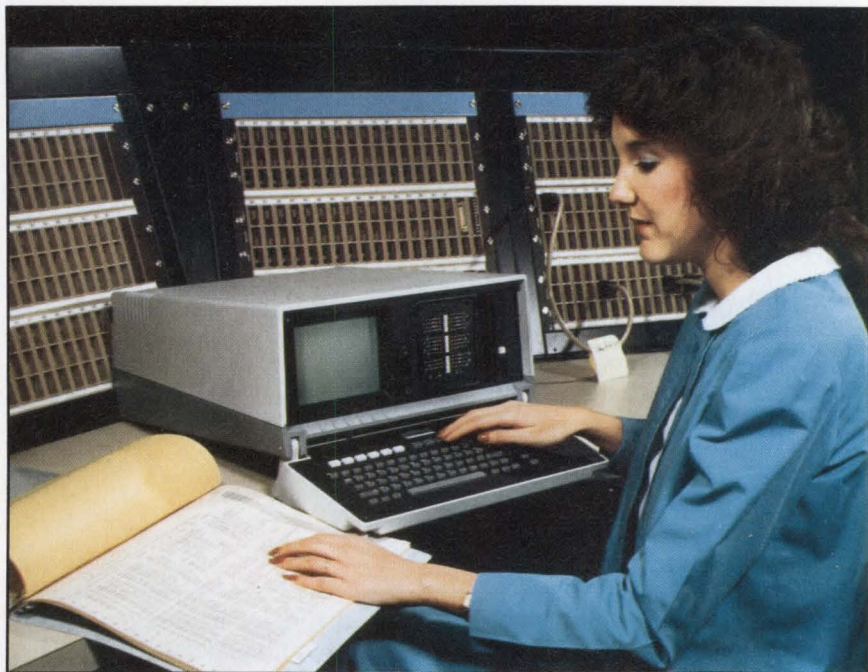
Combining power with simple operation, the Simon 5 protocol simulator/monitor serves as a central console instrument or portable field unit. Diagnostics range from standard bit and block times to response time measurements on SNA cluster controllers.
