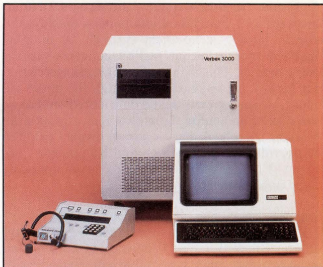
Fig 3 The speech-processing unit measures 22.5 x 23.5 x 26.5 in. The user workstation features a microphone headset the user employs to input verbal data and commands.
