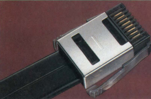
Shielded Data Link connectors available in 4, 8, 16, 24 contact configurations. Insulation-displacing design provides redundant contact on each conductor. Built-in polarization/keying system.
