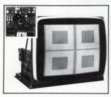
High resolution, VR-Series 20-in. monitors have a horizontal frequency of 31 to 68 kHz. The raster-scan device displays up to 1100 noninterlaced lines refreshed at 60 frames/s. The display runs at a pixel level of up to 100 MHz. At that point, the video has a rise/fall time of 40 ns using either ECL or TTL inputs. It provides 100 lines/in. at 60 Hz or 200 lines/in. in both vertical and horizontal dimensions. **Moniterm Corp**, 7160 Shady Oak Rd, Eden Prairie, MN 55344. **Circle 345**
