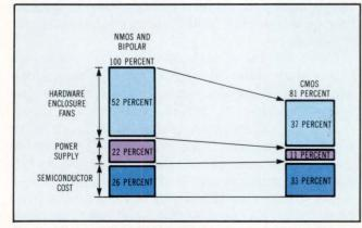
Fig 2 Despite higher semiconductor costs, CMOS reduces overall system costs by decreasing both cooling and power supply equipment.
