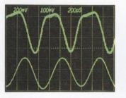
High toggle rate HMD-11141-1 Shift Register showing clock (lower trace) and output functions.
