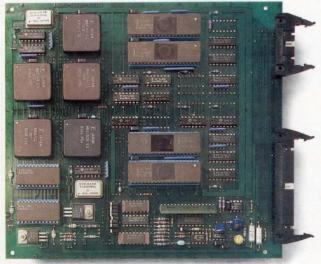
That's why Fujitsu now offers the world's *first* 14,400 bit per second modem card, along with companion 9,600 bps, 4,800 bps and 2,400 bps core modems. All three single PC boards employ custom digital signal processors. And from a standpoint of versatility, the units are compatible with *any* type of equipment.
