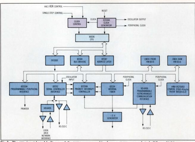
Fig 3 The CPU input board built around the 80C86 processor chip shows a CMOS approach to building a 16-bit processor. This prototype system also features a completely static design and a parallel interface using the 82C55A programmable peripheral interface.
