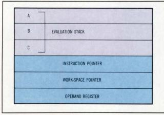
Fig 4 The register set consists of a small set of function specific registers to minimize process swap time and simplify compiler design.
