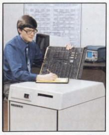
Operating at nearly 1 MIPS, the Harris 60 uses VLSI/LSI circuits, custom gate arrays with over 8000 gates, and a 256-Kbit RAM to decrease bulk. Performance enhancements such as the integrated scientific arithmetic unit (ISAU) increase reliability.
