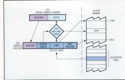
Fig 3 To switch memory references to a new segment, user programs simply load a selector into a register. The 80286 then takes over by loading the rest of the register with all the information needed to perform address translation.
