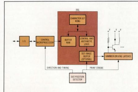
Fig 1 The basic control electronics of a dot-matrix line printer include an I/O section, a control microprocessor, and dot-generation logic (DGL). If a large shift register is used in the DGL, the overall logic is much simpler than in conventional implementations.
