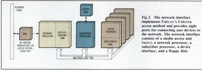
dedicated message because only that unit can use the corresponding message to send information over the network. In contrast, a contention message number is assigned to more than one interface unit. Those units must contend for that message's use. Moreover, each interface unit can have multiple numbers assigned to it.
