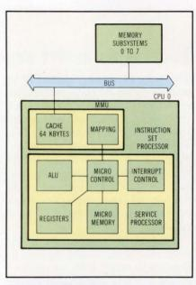
The CPU in Modcomp's 32/85 executes two instruction sets; one compatible with the 16-bit Classic II/75, the other providing 32-bit addressability. The instruction set processor is a complete ALU consisting of a functional microprogrammable processor with hardware multiply and floating point arithmetic. Microinstructions are contained in a writable control store.
