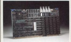
**MLZ-VDC** intelligent 640 x 480 x 4 color graphic controller based on the NEC 7220 controller chip with on-board Z-80 CPU, DMA controller, and user definable FIFO interface to Multibus<sup>™</sup> Users may display up to 16 colors from a 4K palette. Up to 1024 x 1024 x 3 interlaced also available.
