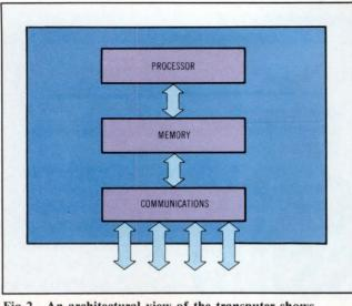
Fig 2 An architectural view of the transputer shows processor, memory, and communications on a single chip.
