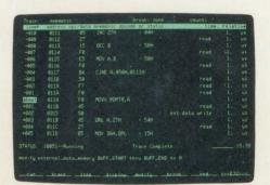
Trace photo of internal data bus is example of how the HP 64264S Emulator shows you more of the 8051 internal operation than ever before.
