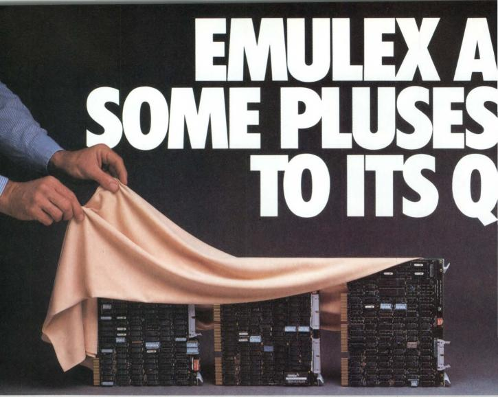
New UC02 emulating host adapter using Mass Storage Control Protocol (MSCP). New CSO2 multiplexer for LSI-11 through 11/23 PLUS and MICRO/PDP-11 computers.
