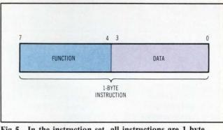
Fig 5 In the instruction set, all instructions are 1 byte long. The 4 MSBs represent a function code and the 4 LSBs are data.
