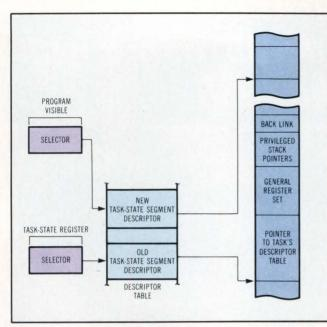
Fig 4 Just as with address translation, programmers are not bothered with the details of a task switch. Instead, after loading the task-state register with the selector to a new task-state segment's descriptor, they let the CPU bring in the information that specifies a task's state. This is contained in the task-state segment.
