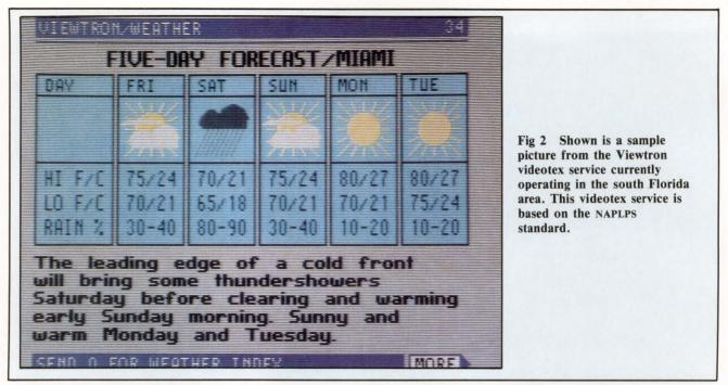
To implement a videotex system, the user needs a terminal; a modem that converts digital to analog; a decoder; and, of course, the transmission lines. The service on a videotex system is usually presented in menu form with the user advancing from a main menu to increasingly more specific offerings. The
