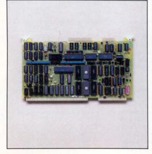
CMX 1600 expansion module, the maximum reaches 160 Kbytes. With a RAM/ EPROM mix, standard onboard capacity is 48 Kbytes, expandable to 80 Kbytes with the CMX module.
