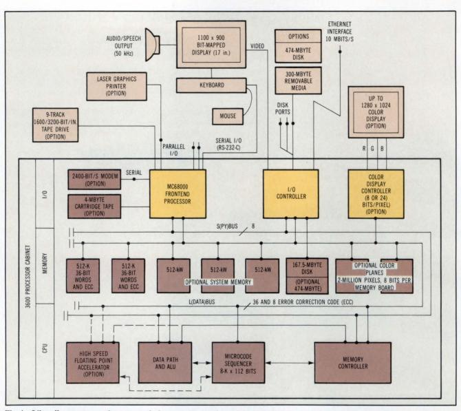
Fig 4 Like all computers, the 3600 symbol processor consists of three sections: CPU, memory, and 1/O. However, the stack-oriented CPU and memory tagging provide an organization specifically designed for Lisp processing.
