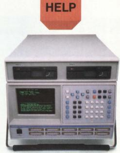
The K105-D gives you two levels of HELP at the touch of a button. First, step-by-step operating instructions that appear along the bottom of the analyzer screen. Second, a menu that allows you to select more detailed "help" should you need it.
