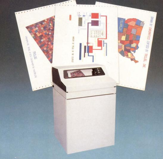
TRILOG's patented multicolor technology provides full color as well as conventional printing on plain fanfold paper at 100 dots per inch resolution.
