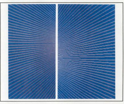
With pixel phasing, a graphics workstation can address portions of individual pixels and eliminate jagged lines. For example, the Merlin 9200 offers an effective resolution equivalent to 3072 x 2304 pixels (left). Using conventional techniques results in vectors as shown on right.
