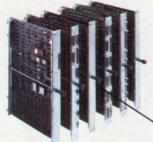
CONFIGURABLE ACCORDING TO USER NEEDS. As many as six processors can be installed in each enclosure. CPUintensive jobs utilize multiple Applications Processors. Systems with heavy disk usage can distribute this load among several File Processors. The number of user ports can be increased by adding more I/O Processors.
