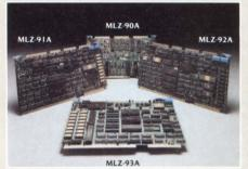
**MLZ-90A** single board microcomputer with nine byte-wide memory sockets for use with RAM or ROM (AM9511 and floppy disk drive controller optional).
