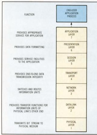
Fig 3 The Open System Interconnection (OSI) model is based on seven functional layers. The NAPLPS standard corresponds to OSI level 6, the presentation level. desired information might be delivered as alphanumeric text, graphics, or a combination of the two (Fig 2).
