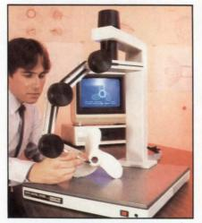
the unit maps fields when sensors for sound, temperature, and radiation replace the standard pointer tip.
