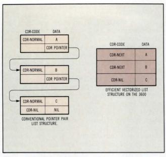
Fig 2 An analysis of Lisp CDR coding, comparing conventional computer architecture Lisp implementations (a) to tagged architecture (b), is shown.
