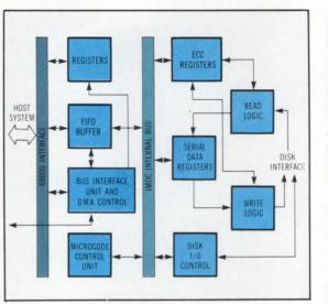
IBM floppy formats. The chip has a DMA controller, and a 128-char FIFO buffer onboard, handles bus arbitration automatically, and uses tables resident in the host's memory to get and send status and control information to and from the host.
