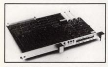
Providing 128, 64, or 32 Kbytes, the MM-6500C employs low power, 8-K x 8 or 2-K x 8 CMOS static RAMS. Three redundant, onboard, parallel, and separately fused backup batteries ensure reliable operation in the event of power failure. Both lithium and NiCad batteries are available. Rechargeable NiCads provide three-month data retention; nonrechargeable lithium batteries permit five-year retention. Realtime calendar/clock provides programmable, periodic, switch-
