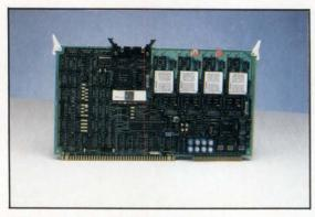
Offering built-in 1-Mbit bubble devices, the FBC504M4M series provides four different memory capacities—128, 256, 384, and 512 Kbytes. The card operates as memory-mapped 1/0 requiring only a 64-byte memory space. Advantages include a single 5-V power source, an internal power fail protection circuit, and data retention even without power.
