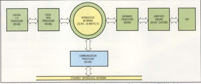
Distributing functions among several processors, the Merlin 9200 increases parallel processing. A 32-bit backplane serves as the network for interprocessor communications.
