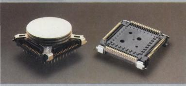
**AMP Low-Height Chip Carrier Sockets:** Duplex plated contacts eliminate solder-bath contamination. Surface-mount or through-hole versions, overall installed height 0.275" for 44-84 positions, 0.350" for 100 positions, to allow 0.500" pc board spacing.
