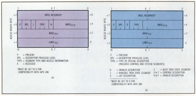
Fig 1 The 80286 segments all operations. To refer to these segments, the CPU uses one type of descriptor for code and data (a) and others for maintaining special structures like those used in multitasking (b).
