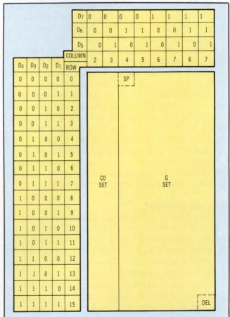
Fig 5 In a 7-bit code environment, the in-use decoding table consists of 128 entries. Here, the table can hold one C-set and one G-set concurrently.
