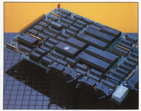
The board relieves the operating system of managing shared disk functions in a networked system through a reserve/ release command. This command manages multiple access to files maintaining data integrity. Moving these functions to the disk controller increases operating system speed and improves file-sharing reliability by simplifying the operating system.
