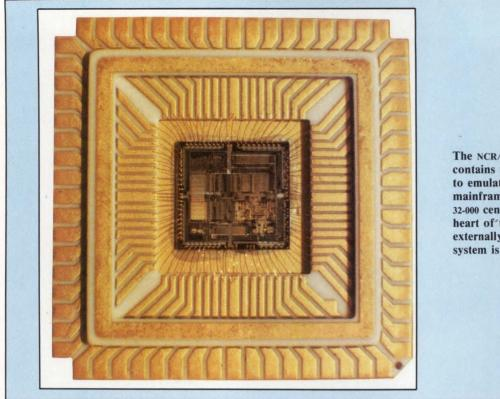
The NCR/32 VLSI processor family contains the only micros designed to emulate existing midrange mainframes. Shown here is the NCR 32-000 central processor chip, the heart of the chip set. This externally microprogammable VLSI system is currently available.
