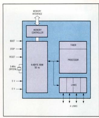
Fig 3 The IMS T424, 32-bit transputer contains a 10-MIPS processor, 4 Kbytes of 50-ns RAM, and four 1.5 Mbyte/s full-duplex communication links. It addresses 4 Gbytes of memory and has an external memory bandwidth of 25 Mbytes/s. Implemented in a 2- $\mu$ m CMOS process, the chip contains 250,000 devices.
