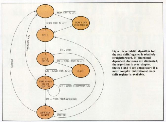
established by the design of the main register is desired. But, this requires additional logic and a supplementary counter programmed with a value that can interrupt the fill algorithm of Fig 6 after the programmed of printable dots passed into the main shift register.
