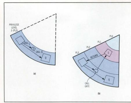
Fig 6 Although 80286 hardware shields programmers from seeing any difference between calling a subroutine Q at one privilege level (a) and using a gate to call a subroutine s at a more trusted level, (b) the mechanisms differ. When the call gate passes control to subroutine s, the gate also passes a copy of the calling subroutines stack to s.
