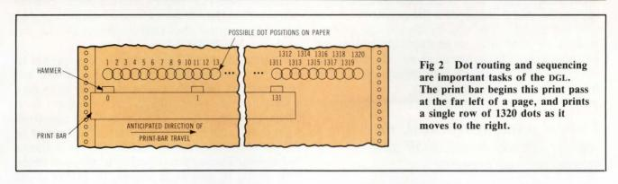
the hammer-driving circuits cannot collectively accept simple raster-scan dot data like a video display unit. For example, as the print bar on a 132-hammer line printer moves from one extreme position to the other, each hammer passes across its exclusive 0.1-in. print area. Each hammer prints as a 0.1-in. mini-raster scan, but the print bar, viewed as a unit, appears as a conglomeration of 132 disjointed raster scans.
