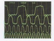
HMD-11016-1 Binary Counter's 2, 4 & 8 synchronous division with 2.0 GHz input. (Input & output data attenuated for presentation purposes.)
