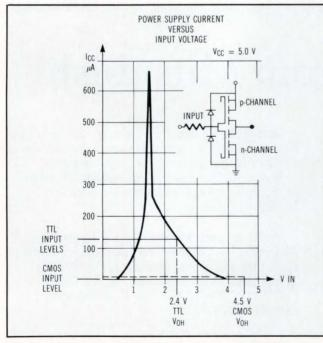
Fig 6 CMOS input circuit transfer characteristics show the danger of allowing the input voltage to float within the active region of the device. The floating inputs will settle at the threshold voltage where current flow is greatest. Consequently, unused inputs must be tied to either  $V_{\rm CC}$  or ground.
