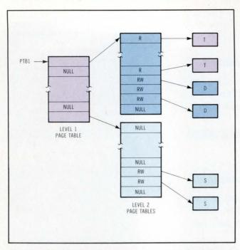
Fig 2 This user process map shows that in the NS16000 memory management scheme, the first-level page table entries point to second-level page table entries, which in turn point to the text (T), data (D), or stack (S) areas. Protection is provided in hardware. Text is read only (R), data is read/write (RW), and the stack is read/write.
