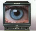
Barco provides a full range of color displays, from 14" to 26," with horizontal scanning systems from 15 to 37.5 Khz, and vertical scanning from 40 to 120 Hz. Choose between standard and high resolution (0.31 dot triad pitch) CRT's with normal and long persistence phosphors, available in both delta gun and the most advanced in-line gun technology. And, of course, Barco is expert at manufacturing to your own specifications and requirements.
