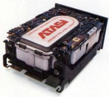
ATASI's 46 Mbyte, 5<sup>1</sup>/<sub>4</sub>- inch Winchester disk drives are available in production quantities immediately.
