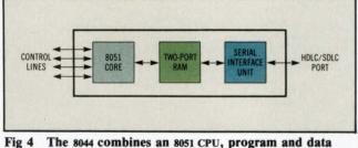
Fig 4 The 8044 combines an 8051 CPU, program and data memory, plus HDLC/SDLC controller on a single chip to build a simple, low cost network station or peripheral.
