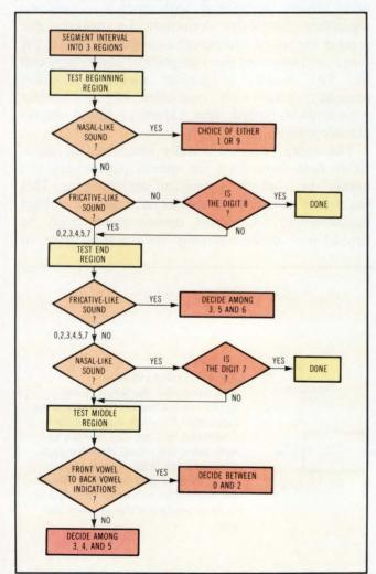
Fig 5 The preliminary decision-making algorithm determines which digit is spoken using input from a sound class generator.
