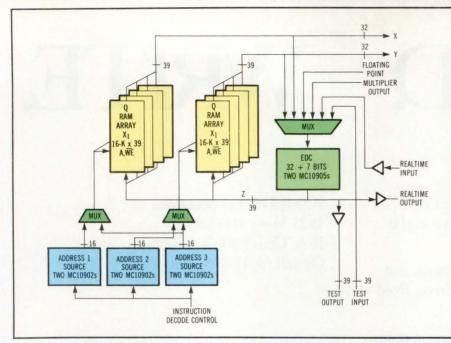
Fig 3 The MC10902 is efficient in operand address generation and arithmetic sections. To access a vector, the unit computes a sequence of locations from initial base address, displacement, index, and step-size values. The MC10905 error detection and correction (EDC) improves data validity and enhances testing diagnostics, yet only increases the pipeline by one cycle.
