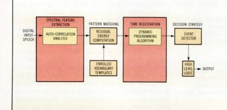
Fig 1 After the analog waveform is sampled, digitized speech input undergoes auto-correlation analysis to perform spectral feature extraction. These features are then matched against stored reference templates, generating a residual energy proportional to the difference between the two feature sets. Dynamic time warping adjusts for speed variations between input and template.
