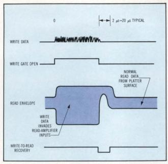
Fig 4 Write-to-read recovery determines how long it takes for the drive's read circuits to recover from high level excitation after a write operation.
