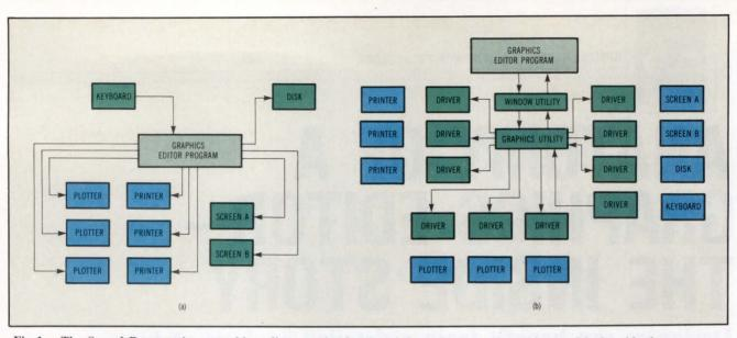
Fig 1 The Sound Presentations graphics editor can be developed from the ground up (a), or with the aid of a graphics tool kit (b). Tools allow a faster time-to-market while custom design offers only incremental technology advantages.
