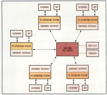
In a star network, such as Spectrum 700, each PC communicates with a central host. The host then mediates all file and message transfers and acts as the central file and print server.
