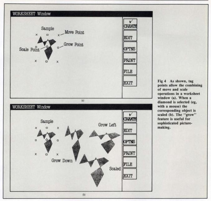
objects such as text, lines, boxes, circles, and polygons (Fig 3). All of these creation processes can be undone with the backspace key. Moreover, each of the worksheet objects can be deleted, moved, scaled, rotated, copied, grouped, or ungrouped. These functions, like the creation functions, can also be undone.
