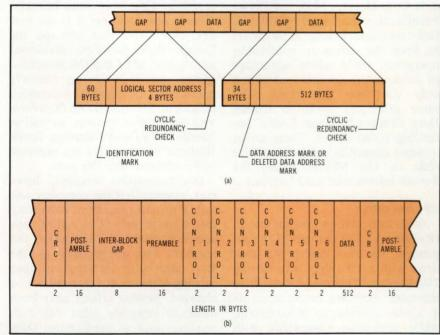
To provide maximum compatibility with existing disk controllers, one option involves using a floppy-style track format with Tandon's TM951 tape drive (a). Contrast this with the more conventional layout of the DEC TK-50 tape cartridge with large control word for file marks and byte counts (b).
