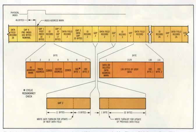
Fig 2 To format a diskette to the IBM 3740 scheme (128 bytes per sector) with a Western Digital controller, a Write command must be issued and the data register loaded with the following: the sector size in bytes, the number of sectors per track, the number of usable tracks, the identification address mark, the side number, the gap sizes, and the step rate.
