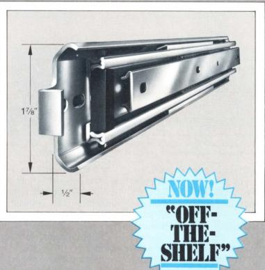
The 4930 is a low cost, ball bearing steel slide rated at 100 lbs. per pair which provides 1" more than full extension and is available with or without mounting brackets.
