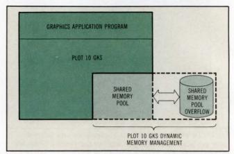
Fig 4 A dynamic memory management facility exists in PLOT 10'S GKS and allows allocation and reuse of a memory pool. When the pool is full, parts are copied to a disk file. The parts copied are intelligently chosen for minimal system impact.
