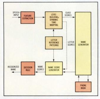
Fig 2 Spoken, spelled names are recognized in this automated directory listing retrieval system. The syntactic rules of the name generator use subsequent input to resolve ambiguities.
