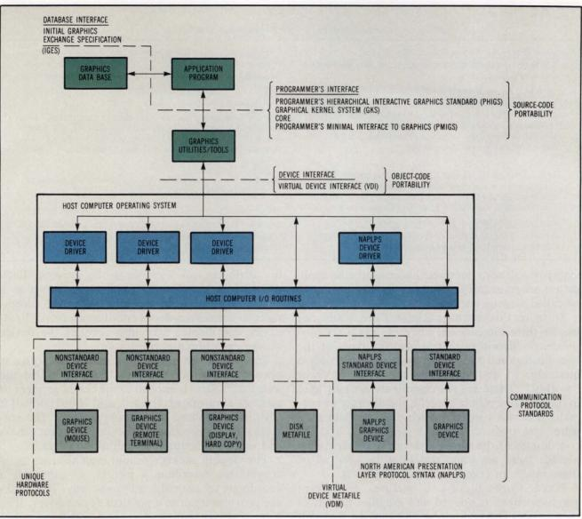
Fig 1 Accepted and proposed national and international graphics standards all have carefully defined software to provide separate, different-functionality interfaces between data bases, programmers, and devices in a graphics-based computer system. The schematic represents relationships, not actual positioning.
