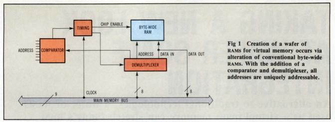
Using this method, a wafer memory operation occurs in several bus cycles: opcode/RAM address, column address, row address, and data. (Note that power dissipation on the wafer is not a problem because all but one of the RAMs on the wafer is in standby mode.)
