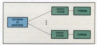
Fig 3 Open system architecture supports host-controlled graphics, distributed network graphics, or a partially distributed system architecture in which major portions of the graphics display pipeline are off-loaded from the host computer.
