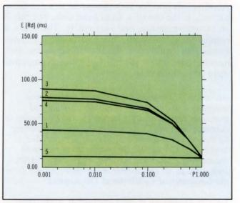
Fig 1 Computer analysis produces mean disk response times of five disk organizations. Plots of disk times converge at the fastest response time-when the probability of no arm movement equals 1.
