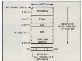
Fig 3 Each Ethernet frame consists of five fields. Destination and source fields indicate where the message is going and from which station it originated. The data field can contain as few as 46 bytes of data and as many as 1500.
