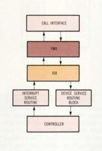
With the I/O and file management (IOX and FMX) extensions to VRTX, calls for services are routed through VRTX to the call interface table. Access to a specific controller is made via a device service routine block, which is also reached via a pointer. IOX can handle multiple devices and channels in this manner.
