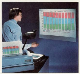
Fig 10 Traditional manual creation of color transparencies can take hours or days depending on complexity, and can cost \$20 and up. With the increased use of color CRT displays, newer photographic techniques have allowed creation of color transparencies in 10 min at a cost of about \$10. ACT claims its ink-jet printer can directly generate computer color graphics in transparency form in 90 s for only \$1.75 each.
