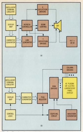
Fig 3 Circuitry for CRT displays (a) differs significantly from that of ac plasma or electroluminescent displays. The required high voltage power supplies also add weight and bulk. The ac plasma and electroluminescent circuits (b) differ mainly in the types of row and column drivers used (SN75500 and SN75501 for the plasma display; SN75551, 2 and SN75553, 4 for electroluminescence), and in waveform generator voltages (100 V for plasma, and  $\pm 200$  V for electroluminescence).
