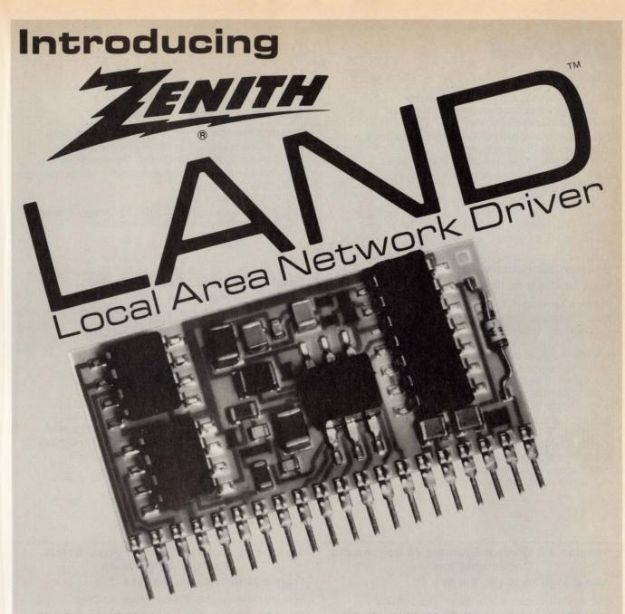
The Zenith LAND Hybrid (Local Area Network Driver) is a cost-effective, highly reliable interface for baseband LAN's including Datapoint's ARCNET™, and other compatible systems.
