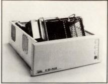
Design allows expansion of an additional 9 full-quad boards, or 19 halfquad boards, or any combination. The basic system is offered with a choice of 256K or 512K bytes of RAM. In one to nine quantity, prices range from \$4465 to \$5265. ADAC Corp, 70 Tower Office Park, Woburn, MA 01801. Circle 305
