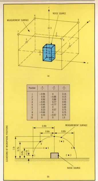
Fig 1 Standard ISO 7779 could feasibly be adopted as an industry standard for measuring acoustic noise in printers. It provides for a sound power measurement, a sound pressure measurement in a bystander position, and clearly defines the test operating conditions. Sound power level can be derived by taking sound pressure readings from either a 9-microphone array in a parallel piped arrangement (a) or from a hemispherical surface with a 10-microphone array (b).
