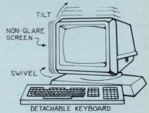
Ergonomics: MPC's terminals offer a non-glare screen, rotate 60° in either direction and compensate for height variations by tilting up to 20°. The detachable keyboard meets European DIN specifications.
