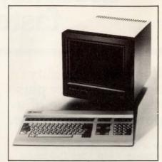
editing, memory and line lock, ASCII comm code, RS-232 interface, and transmission rates from 50 to 19.2k baud. The terminal is priced at \$1085. Beehive International (UK) Ltd, Index House, Ascot, Berkshire, SL5 7EU, England. Circle 408
