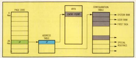
The VRTX/80 is entered by a restart (RST 5) instruction that jumps to location 28 Hex in the Z80's page zero. This location must contain a jump (JP) instruction to the first byte of an address table, which in turn, contains a jump to the VRTX internal entry point, and a pointer to a configuration table.
