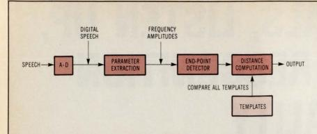
Fig 1 Template-matching speakerdependent word recognizers are best suited for single-user data terminals. Users must "train" the system to recognize their voices by making templates of their voice patterns. Such templates are used by the system to make comparisons with spoken voice patterns.
