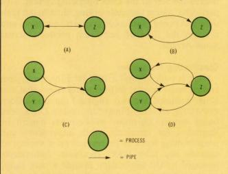
next process reading that file). A pipe is a conduit with two ends, each of which is attached to a different process. One end appears as a write-only file, the other as a read-only file. The Figure shows four typical pipe uses.
