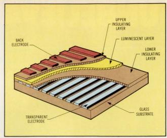
Fig 2 Electroluminescent panels use doped zinc sulphide that emits light when the voltages, which the embedded electrodes impose across it, exceed a threshold value.
