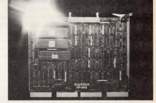
Q-Bus. And Quest memory is available in static RAM (90 nsec cycle—no need for cache) or dynamic RAM; both on quad boards for up to a maximum of 16 MB.
