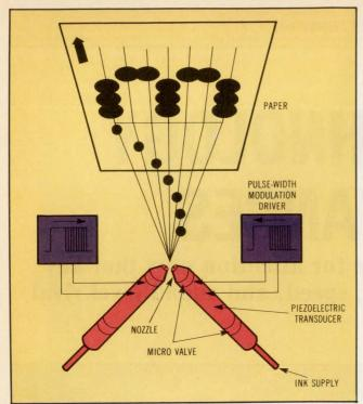
A growing problem for ink-jet printer manufacturers has been the low reliability of the ink jets themselves. To increase reliability, jet number must be reduced. NEC's drop collision deflection technique uses only two jets to emit two simultaneous drops which, upon colliding, combine at a point adjacent to the nozzle orifices. Micro valves apply a constant pressure on the ink; pulse-width modulation drivers control the direction of the ink drops.
