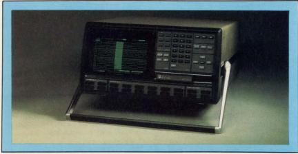
triggering helps to isolate problems and unravel machine code. Another timesaving feature is the monitor, which follows instructions and execution and tells the user what went wrong and how to correct it.
