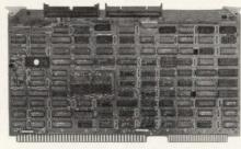
Xylogics 472 Multibus Tape Peripheral Controller.
