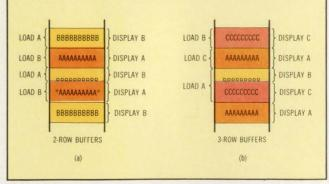
Fig 3 For split-screen scrolling applications, a character row could be displayed for only a single scan line. With two row buffers (a), this does not leave enough time for the reloading of the alternate row buffer, which results in a flashing screen. With three row buffers operating in a rotating fill-display mode (b), any single row buffer can be displayed for one scan line without any danger of screen flashing.
