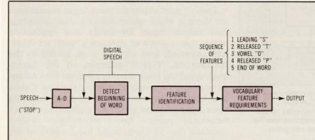
Fig 2 Speaker-independent word recognizers are phonetically based, that use no templates, and require no user training. Operating on the principle of feature identification, speaker-independent systems need less memory than speaker-dependent types, making them more cost-effective for data terminals.
