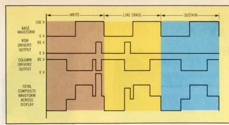
Fig 6 The base waveform establishes the basic timing and voltage levels for writing and erasing ac plasma displays. Signals applied to the row and column drivers determine whether data will be written, erased, or sustained.
