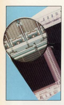
Speed is often an important factor in a memory device. In a view of this, the Am27256 is a 256K-bit UV EPROM with access times down to 170 ns. Also, the memory chip features redundancy, a fast programming time, and an autoselect mode.
