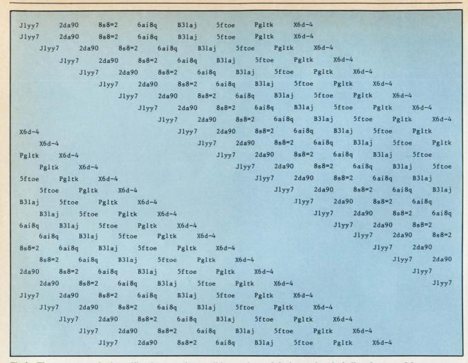
Fig 2 The ISO 7779 standard specifies the operating conditions to be used during testing, including the type of font, paper size and type, line spacing, and print speed. Furthermore, a print pattern specific to the printer's line length is defined. This pattern is for printers that have upper- and lowercase capability and can generate copy with more than 110 print columns.
