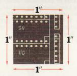
The board section above is for a Burroughs computer using TTL and ECL devices, some packaged in pin grid arrays. 4 mil wire is routed on a 14 mil grid, with three wires between holes. Component density exceeds 2.5 DIPs per in. sq. (14-pin DIP equivalent).
