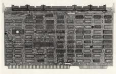
Xylogics 450 Multibus Disk Peripheral Controller.
