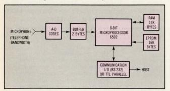
Fig 4 An 8-bit microprocessor and a communications port form the core of Voice Control Systems' speakerindependent word recognizer. Because it operates on the principle of feature identification, this recognizer uses far less memory than speaker-dependent word-recognizer systems.
