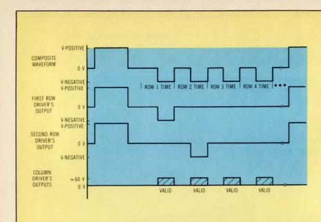
Fig 4 The composite waveform across an electroluminescent display reflects the information on each row driver, with a refresh pulse that maintains an average dc value of 0 V across the display.
