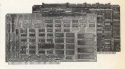
Xylogics 440 Multibus Disk Peripheral Controller.
