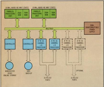
Fig 2 Multiple high speed links separate processor clusters so that interrupted tasks can be easily transferred in this redundant architecture implemented by Auragen Systems.
