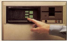
The 1722A instrument controller was designed with industrial applications in mind. This 16-bit microcomputer-based system is optimized for automating factory test and process control systems. It is particularly well suited for applications in which unskilled personnel operate complex systems.
