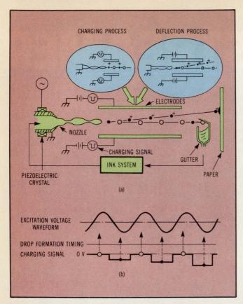
Fig 2 Hitachi's microdot printing technique controls the dot's size and shape by having the ejected ink stream pass from the nozzle between two electrodes used as deflection plates (a). Dot size is controlled by applying a variable excitation voltage that stabilizes the formation of an optimal dot pattern (b). Microdots alternate with large drops, and charged microdots are deflected to the paper while uncharged drops fall into the gutter.
