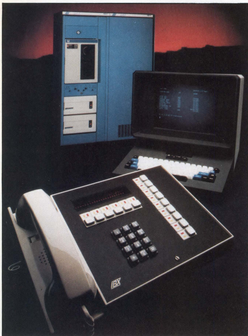
InteCom's LANmark network, based on use of the company's star architecture IBX S/40 integrated business exchange, provides simultaneous voice and data transmission through each of 8192 ports. Interconnection of the 512M-bps Ethernet compatible system is via 2-pair telephone wire.
