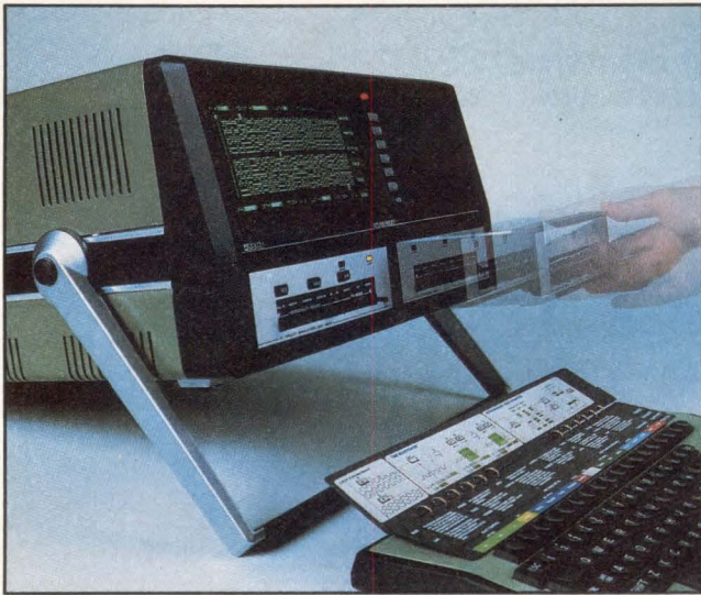
The Dolch Atlas 9600 system can accept 2 plug-in preprocessors in its mainframe and control 12 others, be they logic analyzer, trace, emulation, or word generation modules. The flip chart on the keyboard relates soft key definition to the various modules.
