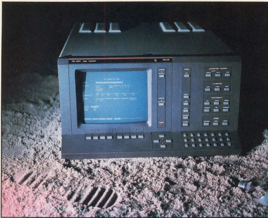
The Philips PM 355. The soft keys in a row along the bottom of the screen are defined by a label at the bottom of the display to guide the user through setup and measurement procedures.
