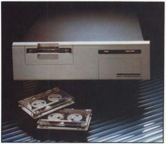
A 31.2M-byte Winchester system, the DSD890 from Data Systems Design, includes a quarter-inch tape backup. The DEC-compatible system replaces more expensive equipment that uses half-inch tape for backup. Its Winchester drive can replace a system that uses three cartridge disks.
