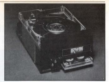
The Irwin 516 subsystem includes a 16M-byte Winchester drive and cartridge tape backup. Fitting a standard  $5\frac{1}{4}$ " configuration, the unit claims high storage capacity on a single platter. Average access time is under 35 ms including move and settling times.
