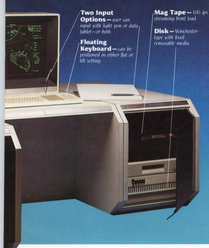
2Kbytes track buffer, 16Kbytes rogram and data memory, and eparate DMA to the floating point processor for instantaneous screen esponse requiring disk access. **Communications Processor** upports all communications to he outside world; system peripherals such as plotters, line printers and phototypesetters, ynchronous and asynchronous lata communications and proto-
