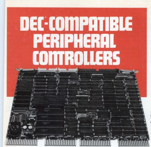
LSI-11<sup>®</sup> compatible controller for 80-300MB SMD and Winchester drives from CDC, Ampex, and Fujitsu
