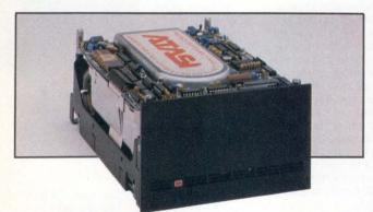
Compact  $5\frac{1}{4}$ " Winchester disk drives from Atasi offer up to 46M bytes of storage capacity. Another advantage of the Series 3000 units is a 30-ms access time, which rivals the speed of larger 8" and 14" drives.
