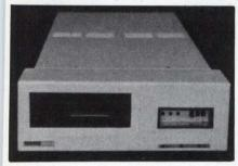
MDP-11 microcomputer system has builtin LSI-11 microcomputer, hard and floppy disk, or cartridge tape system. Disk and tape systems are compatible with std DEC RL01/02, RX01/02, and TM-11. 4M-byte direct addressing is provided. RT-11, RSX-11M, and RSTS-11 operating systems are accommodated. Either 0.5M- or 20M-byte removable media and 5M- or 10M-byte hard disk are provided. MEDICOM/Medische Elektronica en Computer Systemen, Postbus 2070, 2800 BE Gouda, The Netherlands. Circle 307
