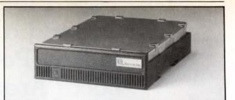
Half-height  $5\frac{1}{4}$ " drives from Disctron store 25.5M bytes (model 620) or 42.5M bytes (model 640). Both versions have a 40-ms average access time. Head positioning employs voicecoil and closed loop servo technology.
