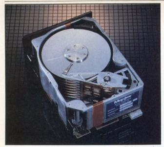
A new  $5\frac{1}{4}$ " Winchester from Maxtor packs 140M bytes of storage on eight stacked disks. The xT-1140 is the latest in a family of  $5\frac{1}{4}$ " drives that have the motor inside the spindle, thus allowing more disks to be stacked within standard physical dimensions. Access time is a low 30 ms.
