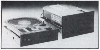
A half-height 5¼" Winchester from Seagate Technology is the first of its class to use thin-film media for added durability. The ST206 (left) is compared with a Seagate standard-height unit. Both drives store 6.38M bytes of unformatted data. The ST206 has an 85-ms average access time and is fully compatible with the widely accepted ST506 interface standard.
