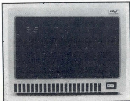
System 86/330 microcomputer. Entire system including disc peripherals is contained in single 21 x 16 x 12" (53 x 41 x 30-cm) cabinet that can be desktop or rackmounted. Package meets UL, FCC, VDE, and CSA safety and emi/rfi specifications
