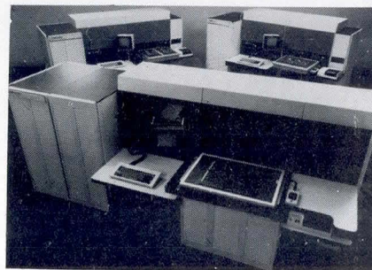
227X circuit board test system family. 2272 (foreground), 2271 (background right), and 2270 (background left) share same basic system architecture and can use same test programs. Fixtures are upward compatible between systems
