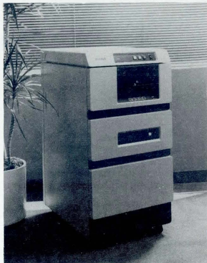
System is designed to optimize UNIX operating system developed by Bell Laboratories. Typical 8-user Plexus P/40 has 512k bytes main memory, 72M bytes disc storage, 8-channel ICP, and 9-track tape unit
