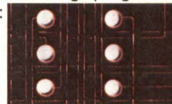
A typical example of the circuit density achievable with Multiwire circuit boards.
