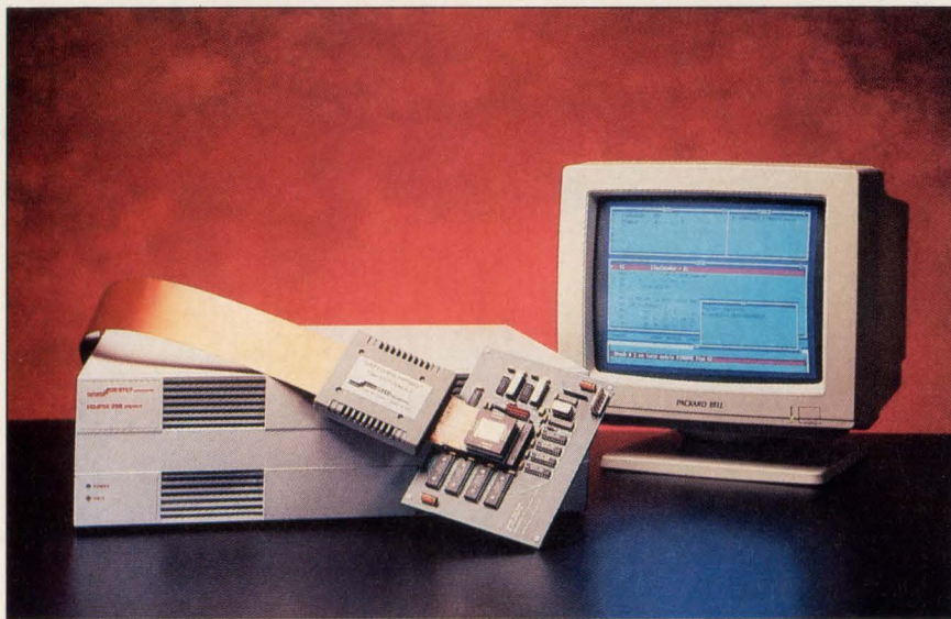
While early RISC tools were poor, most designers admit the tools are getting better. Tools like this 29000 "Eclipse" emulator from Step Engineering are key to the design of successful embedded projects. Among other things, the Eclipse lets the designer examine processor execution statistics, including interrupt latency, instruction cache efficiency and event timing.
