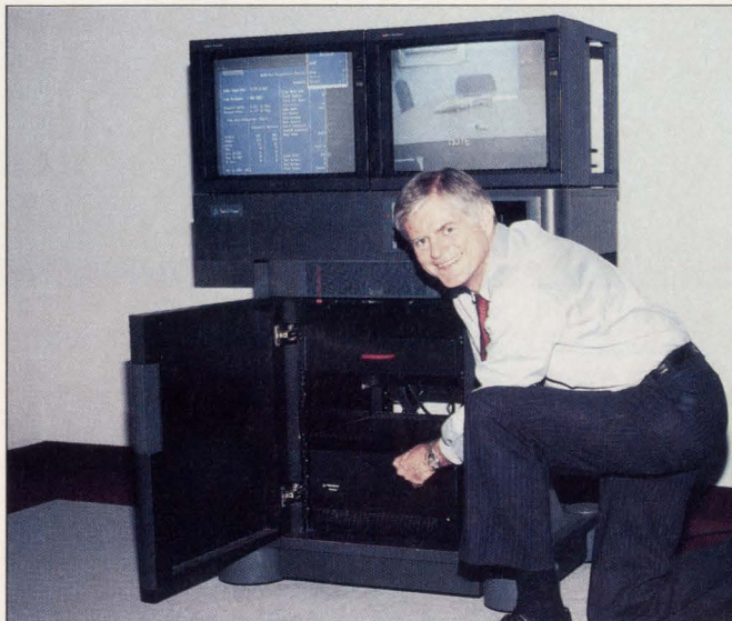
The image processing heart of VideoTelecom's video teleconferencing system is a board using three Intel i960CAs and a custom coprocessor. A fourth i960CA was used in the system as a communications controller. A 386 PC-class machine lets the user incorporate PC-generated material during a teleconferencing session.
