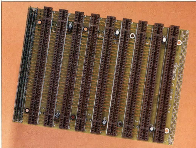
Ziatech's ZT 32B is the first STD 32 backplane on the market. It accommodates both older STD 80 and newer STD 32 boards, allowing 8-, 16- and 32-bit data transfers.
