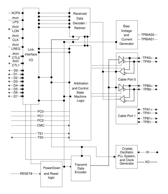
Figure 2. Internal PHY Block Diagram
