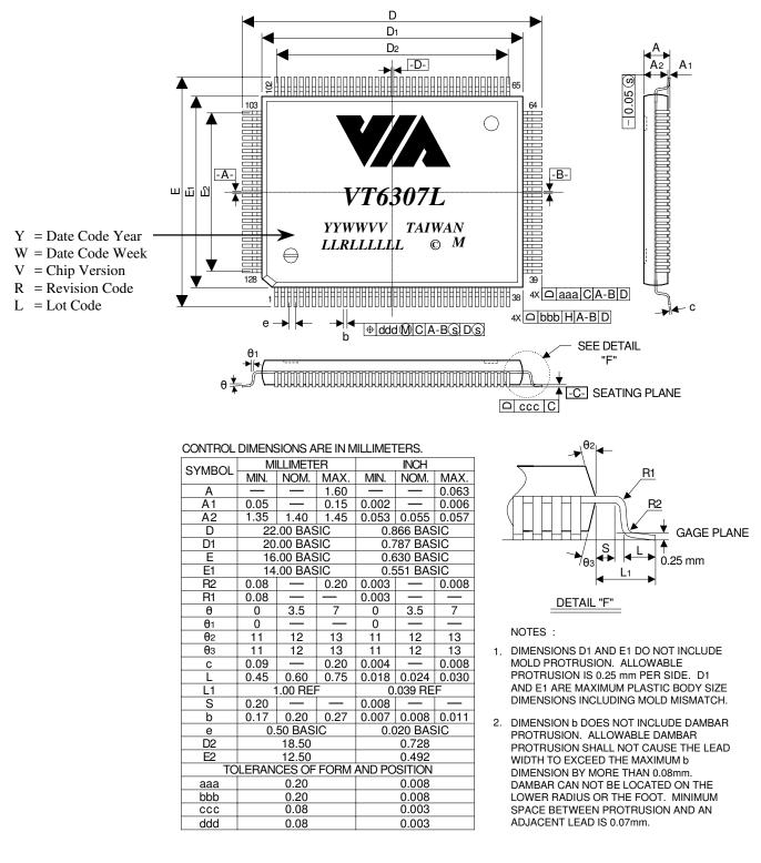
Figure 8. Mechanical Specifications - VT6307L Rectangular 128-Pin LQFP Package
