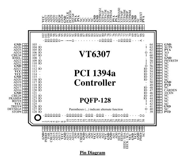
Figure 3. VT6307 1394a Controller PQFP - 128 Pin Diagram 14x20 (Top View)
