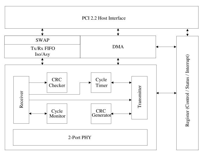
Figure 1. Chip Internal Block Diagram
