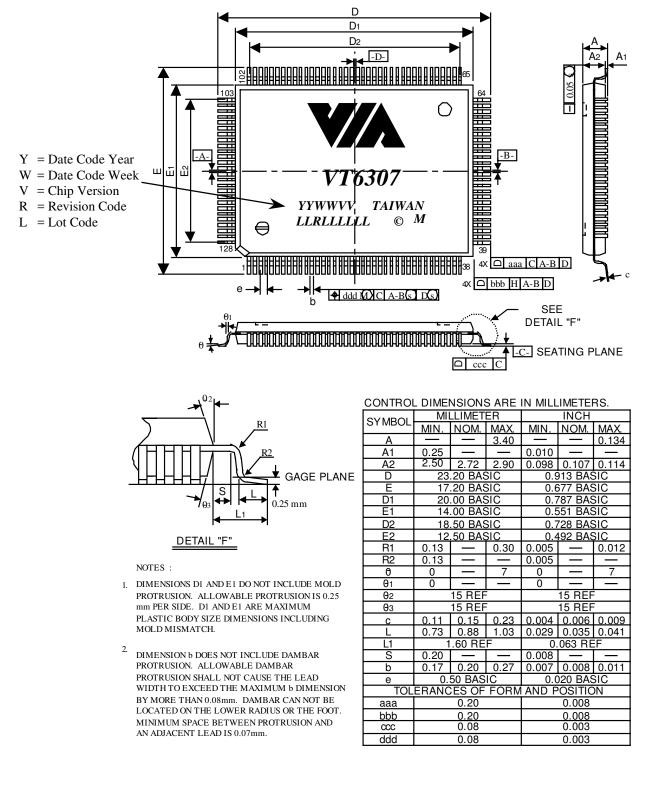
Figure 7. Mechanical Specifications – VT6307 Rectangular 128-Pin PQFP Package
