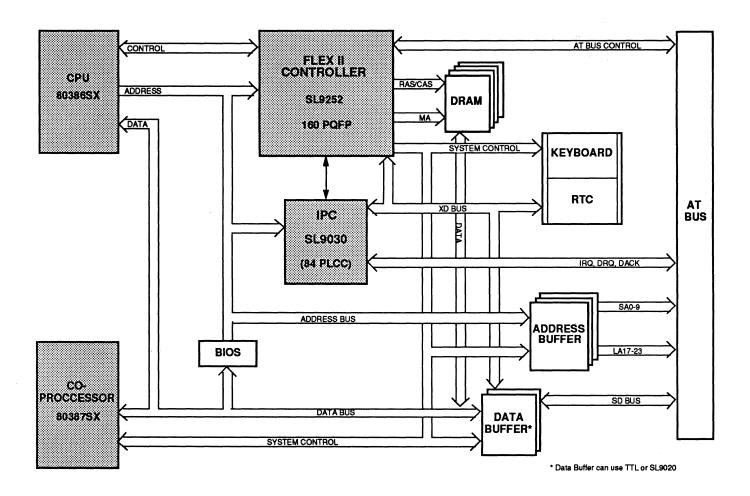
Fig. 1. Block Diagram for 80386SX CPU Board
