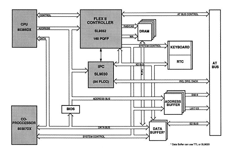
Fig. 1. Block Diagram for 80386DX CPU Board
