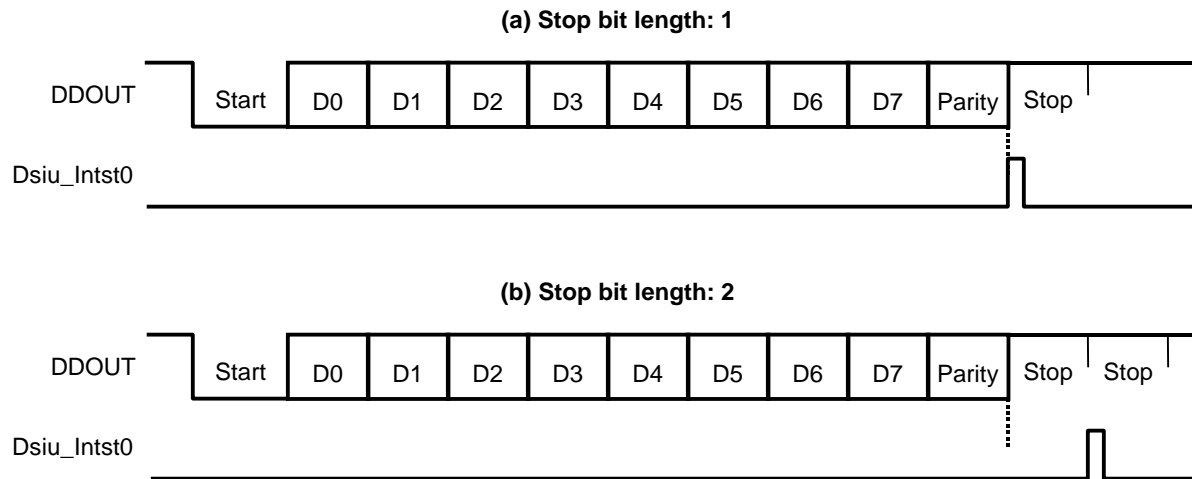
Figure 22-2. Transmit Complete Interrupt Timing
