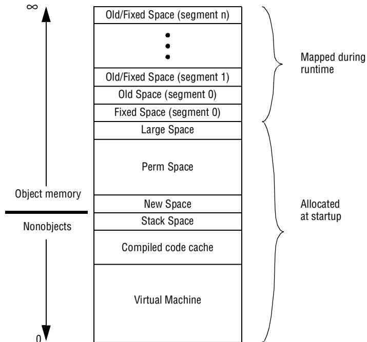
The diagram shows organization of the address space that belongs to a VisualWorks process, with code, non-objects, and the fixed portions of the object memory in the lower portion of the space, and the dynamic spaces and segments of the object memory above.
