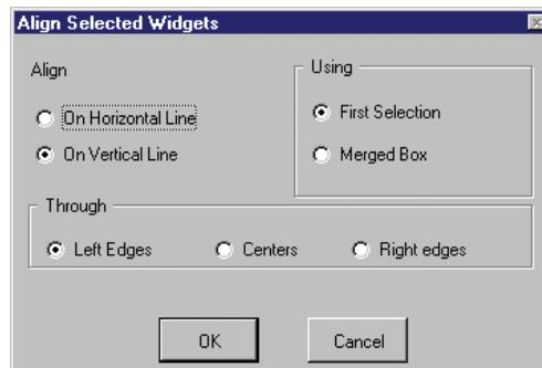
When painting a canvas, you frequently need to make several widgets align along a vertical or horizontal line to give a neat, regular appearance. For precise control you can use the Align dialog, shown above and described below. There are also a set of alignment buttons on the Palette, giving quick access to the alignment functions. You can also use the **Position** properties page to precisely position widgets, but would usually choose to do so only due to scaling consideration
