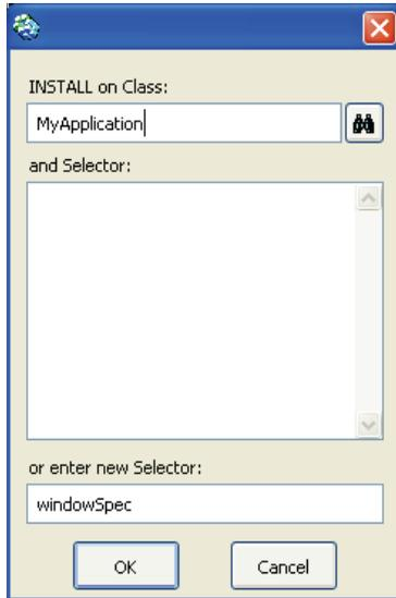
For a new canvas, you need to enter a class name in the **Install on Class** field. This can be a new class name or the name of an existing class. For a new class, you will be asked for the appropriate superclass in a subsequent dialog.
