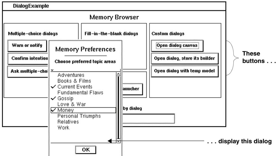
When a standard dialog is not sufficient, you can create your own using the canvas tool. You can then open the interface specification in a dialog window.
