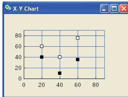
An XY chart indicates any correlations between two characteristics derived from the scattering status of points plotted in the chart.
