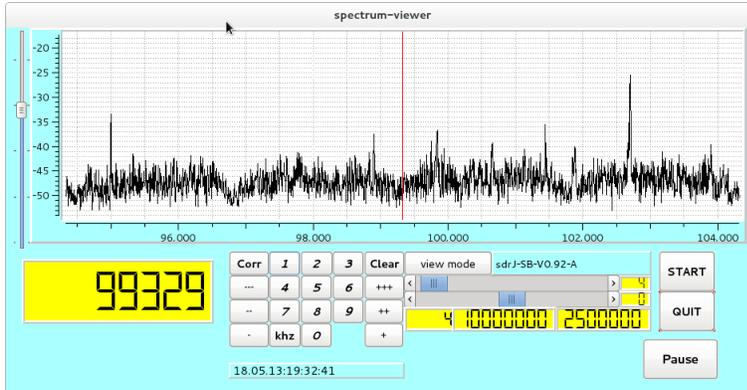
More or less as a gadget, a simple spectrum viewer is added to the set. With this viewer it is possible to view a large spectrum, built up from a sequence of spectra from subsequent frequencies.
