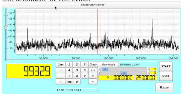
The picture above shows the GUI of the spectrumviewer. Although a gadget, it is interesting since it may give an overview over a pretty large frequency range. Of course, when having selected e.g. 15 Mhz as area, details are lost.
