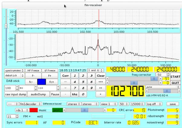
The above picture shows the GUI of the FM receiver. At the top display a spectrum of over 2M is shown, the second display shows the spectrum of the demodulated signal. It can be seen that the GUI of the DAB receiver is simpler than that of the FM receiver, the latter has more settable parameters. One of its advantages is that it can be used to derive the frequency offset in the oscillator of the stick.
