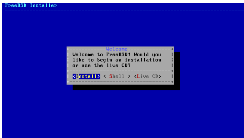
Figure 2-3. Selecting Installation Media Mode
