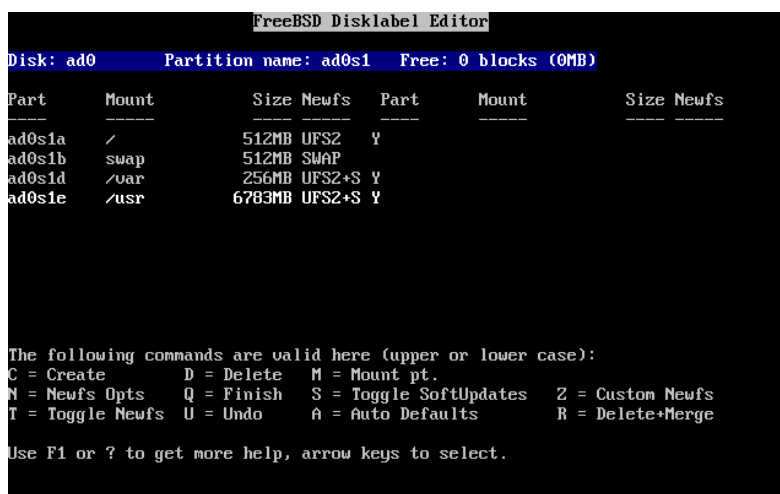
Figure 3-24. Sysinstall Disklabel Editor
