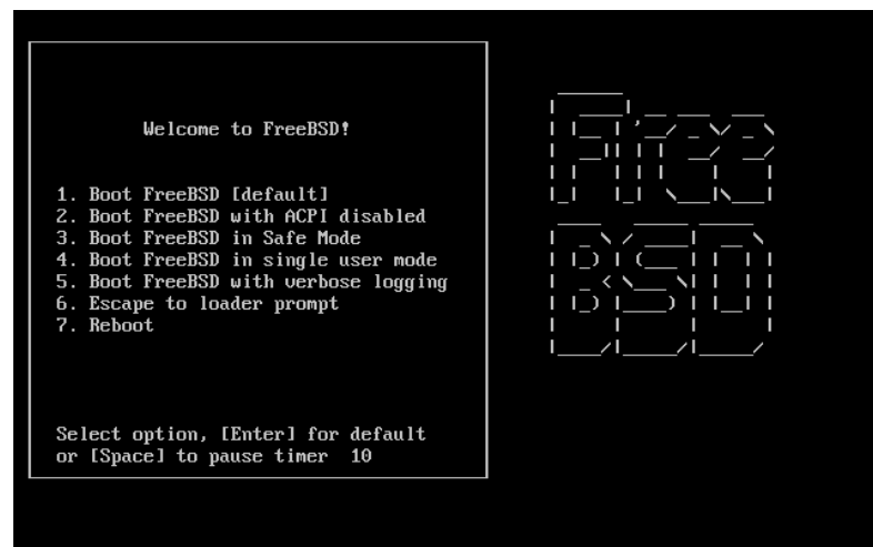
Figure 3-1. FreeBSD Boot Loader Menu
