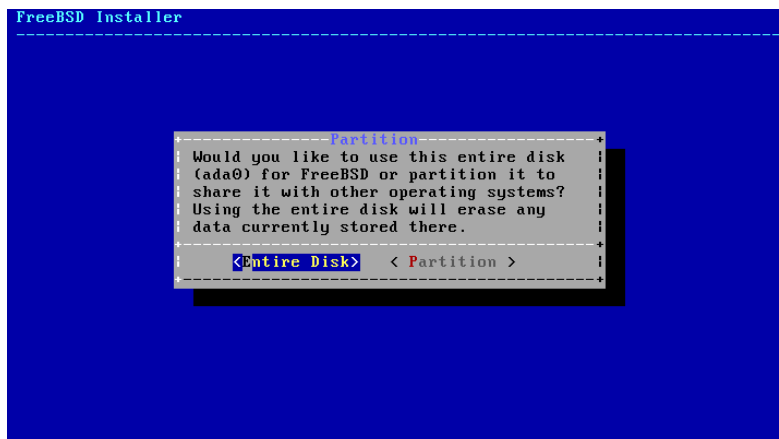
Figure 2-12. Selecting Entire Disk or Partition
