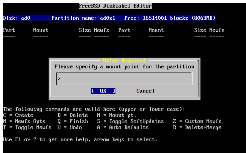
Figure 3-23. Choose the Root Mount Point
