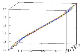
Figure 21.6: Example finite element model the showing triangular elements. The height of each vertex corresponds to the solution value.
