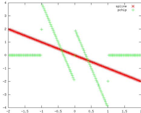
Figure 28.2: Comparison of the second derivative of the 'phcip' and 'spline' interpolation methods for a step function
