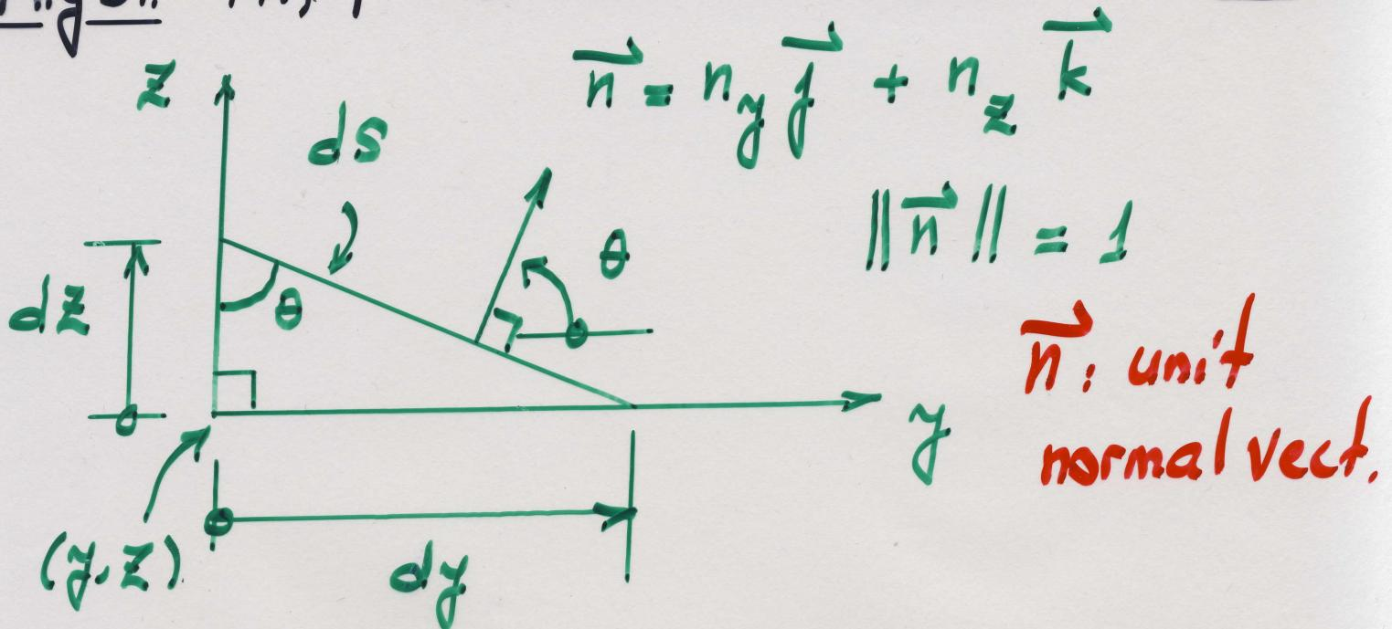
$$\left\{ \begin{array}{l} dz = ds \cdot \cos \theta \\ dy = ds \cdot \sin \theta \end{array} \right. \quad \left| \quad \left\{ \begin{array}{l} n_y = \cos \theta \\ n_z = \sin \theta \end{array} \right. \right.$$
