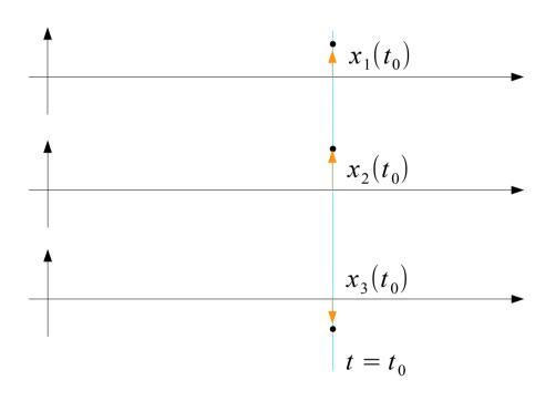
$$E[X(t_0)] = \int_{-\infty}^{+\infty} x f(x; t_0) dx = \mu(t_0)$$
