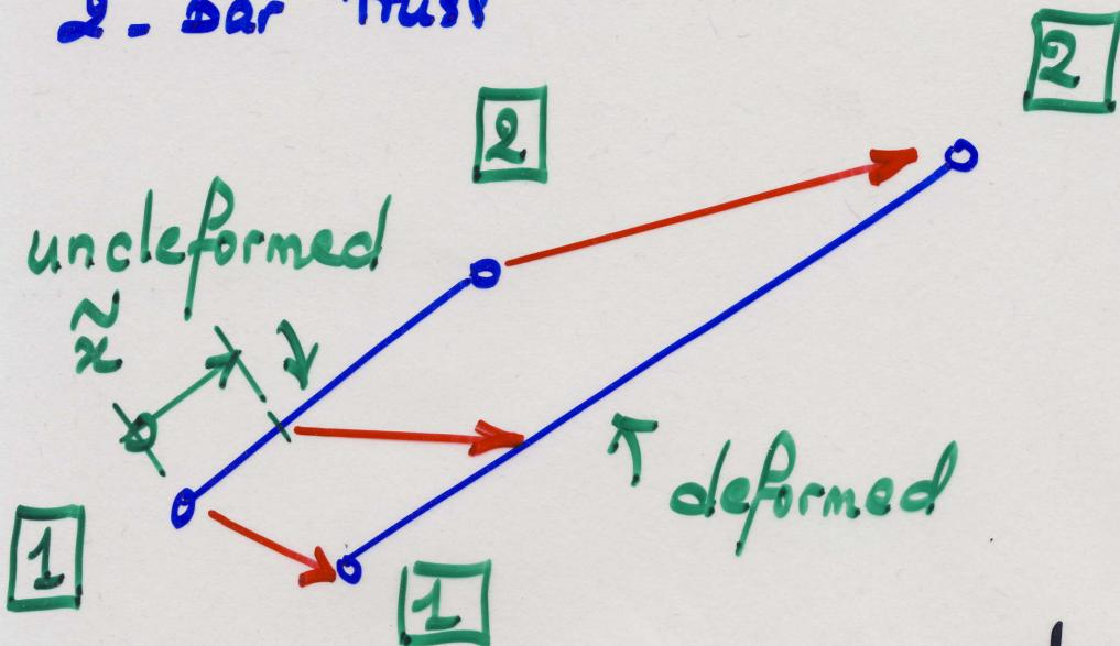
Deformed shape is a straight line, i.e., there was an implicit assumption of linear interp. of disp. betw. 2 nodes.
