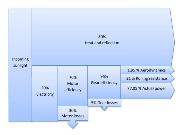
Actual power is again the energy that is used to move the car. This is no wasted energy.
