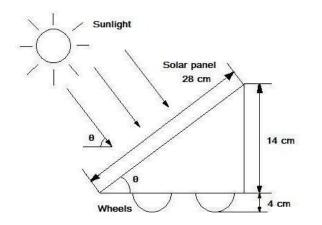
Maximum velocity at the maximum power:  $V = P_{real} / F_{wheel} = 4,31 / 1,19 = 3,43 m/s$
