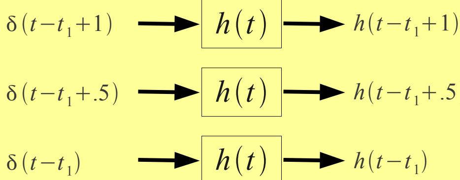
A block diagram of the LTI system. An input signal enters a block labeled  $h(t)$ , which then produces an output signal  $y(t)$ .
