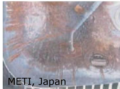
pitting corrosion of X90CrMoV18 in an E10 gasoline blend
