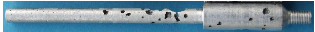
„dry“ alcoholate corrosion of a cast Al-alloy in an E10 gasoline blend
