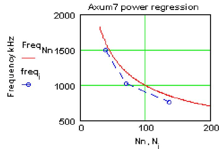
**Axum7 power regression curve - Gillette stainless blade AM diode demodulator given observed (blue dash points) AM station frequency kHz vs number of induction coil turns (Nn)**
