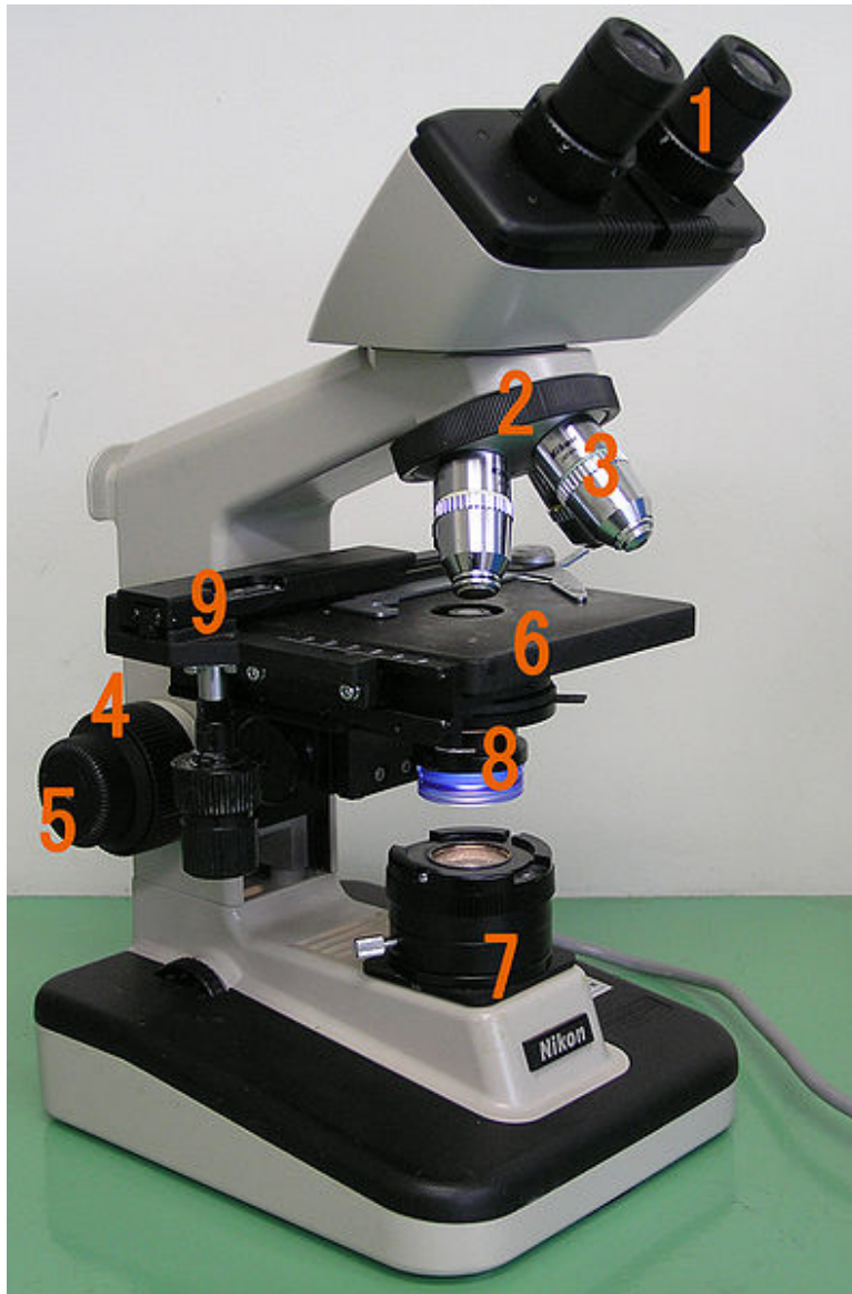
Figure 1.17: Basic light microscopes opened up a new world to curious people. 1, ocular lens or eyepiece; 2, objective turret; 3, objective lenses; 4, coarse adjustment knob; 5, fine adjustment knob; 6, object holder or stage; 7, mirror or light (illuminator); 8, diaphragm and condenser. (11)
