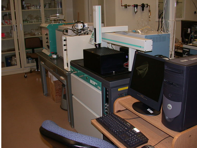
Figure 7.31: The most reliable way to figure out the earth's age is to measure the radioactivity of certain minerals found in rocks (called radiometric dating). This mass spectrophotometer can also be used to measure age of fossils from the level of radiation in minerals surrounding the fossil. (1)
