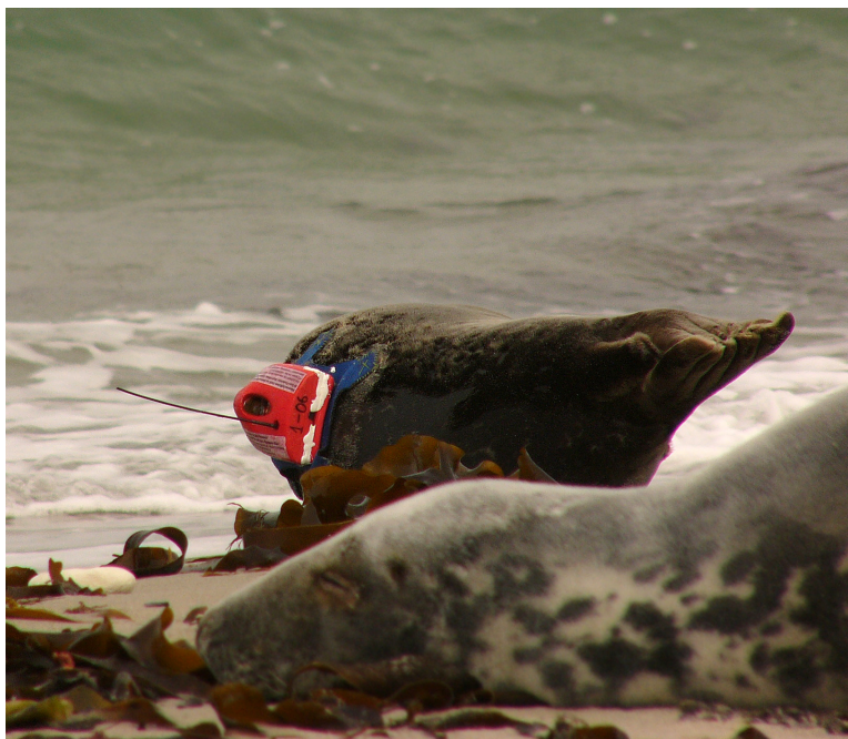
Figure 1.22: A radiotelemetry device used to track the movement of seals in the wild. (22)
