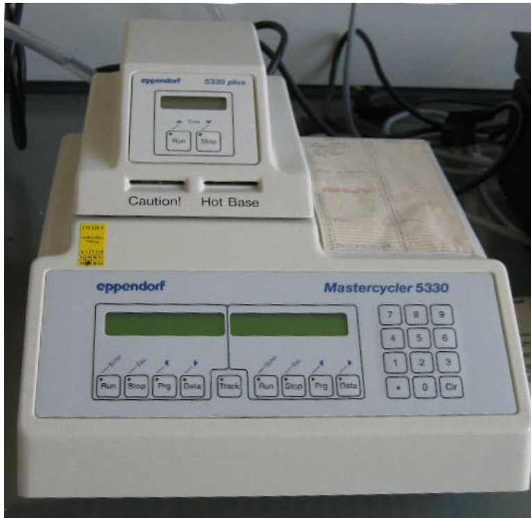
Figure 1.23: A thermocycler used for molecular biological and genetic studies. (17)
