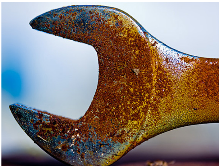
Figure 2.9: Rust is the result of a chemical reaction between iron and oxygen. (16)
