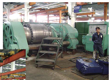
Group of benches of test of valves
