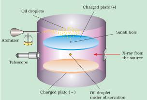
**Fig. 2.3** The Millikan oil drop apparatus for measuring charge 'e'. In chamber, the forces acting on oil drop are: gravitational, electrostatic due to electrical field and a viscous drag force when the oil drop is moving.
