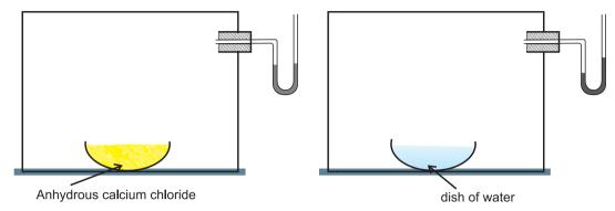
Fig.7.1 Measuring equilibrium vapour pressure of water at a constant temperature
