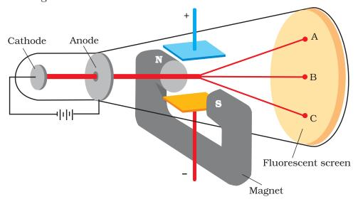
*Fig. 2.2* The apparatus to determine the charge to the mass ratio of electron
