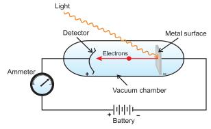
**Fig.2.9** Equipment for studying the photoelectric effect. Light of a particular frequency strikes a clean metal surface inside a vacuum chamber. Electrons are ejected from the metal and are counted by a detector that measures their kinetic energy.
