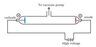
Fig. 2.1(a) A cathode ray discharge tube
