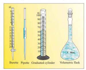
Fig 1.7 Some volume measuring devices
