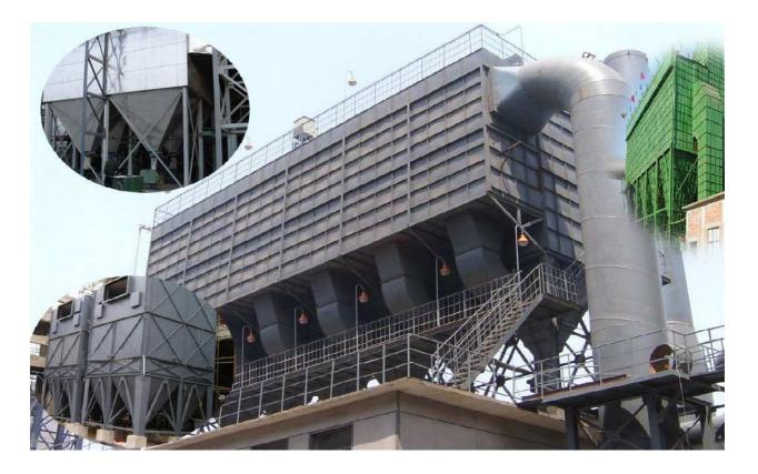
Bag and reduce SO2 dust collector, can also supply water membrane dust collector
