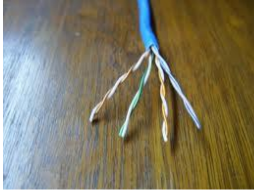
Figure 4: Stripped sheath of the cable
