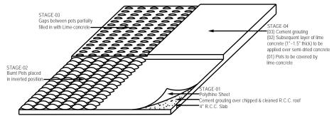
ORTHOGONAL VIEW OF THE ROOF SHOWING CONSTRUCTION OF ROOF INSULATION IN 4 STAGES
