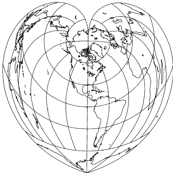
Figure 46C.—Werner projection, with shorelines, 30° graticule. Central meridian 90° W. Polar limit of Bonne projection.
