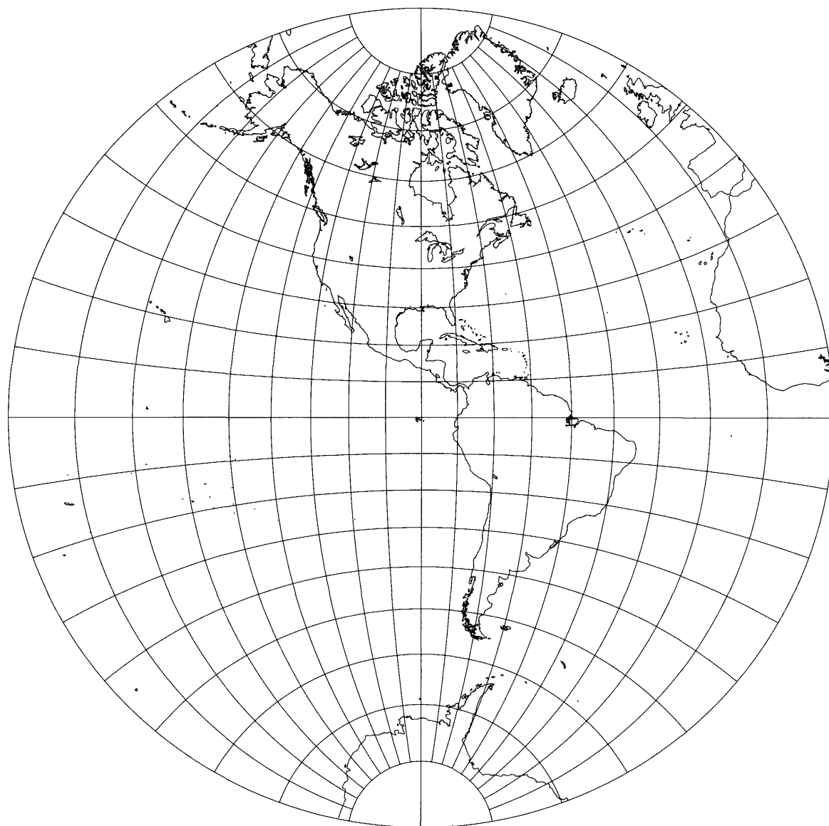
Figure 49C.—Equatorial Stereographic projection, with shorelines, 10° graticule. Central meridian 90° W. Range 90°.
