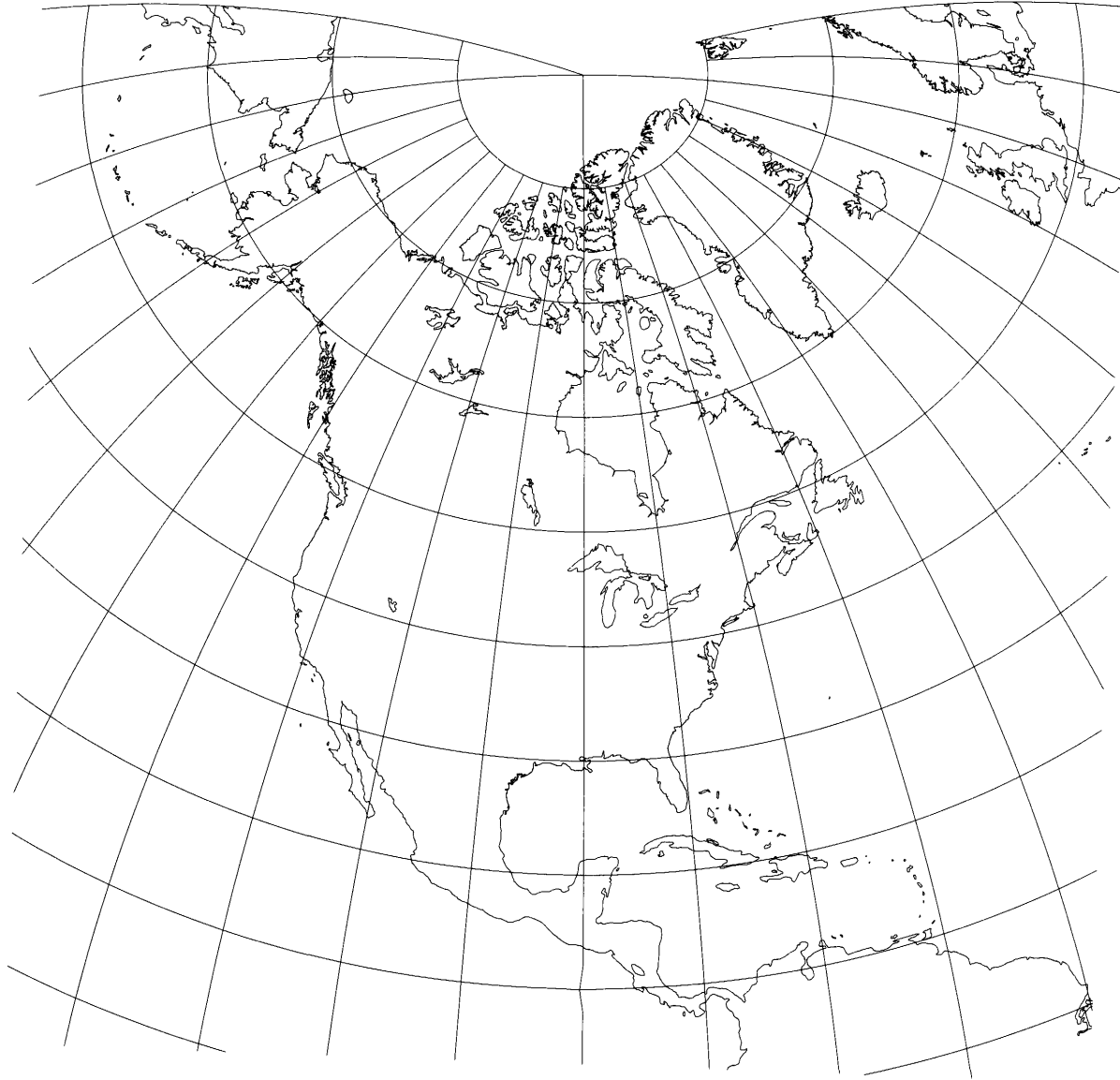
Figure 69B.—Chamberlin Trimetric projection of North America with national boundaries, 10° graticule. Three source points for this map, as selected by the National Geographic Society: (1) latitude 55° N., longitude 150° W.; (2) latitude 55° N., longitude 35° W.; (3) latitude 10° N., longitude 92°30' W.
