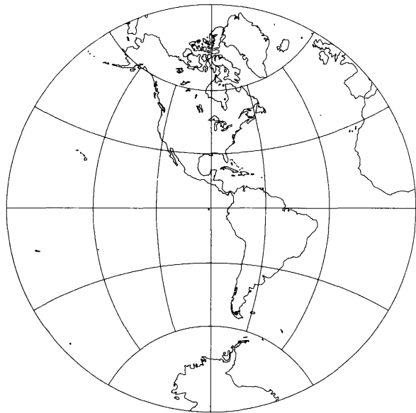
Figure 76D.—Equatorial Stereographic projection, with shorelines, 30° graticule. Central meridian 90° W. Special case of Lagrange with hemisphere in circle.
