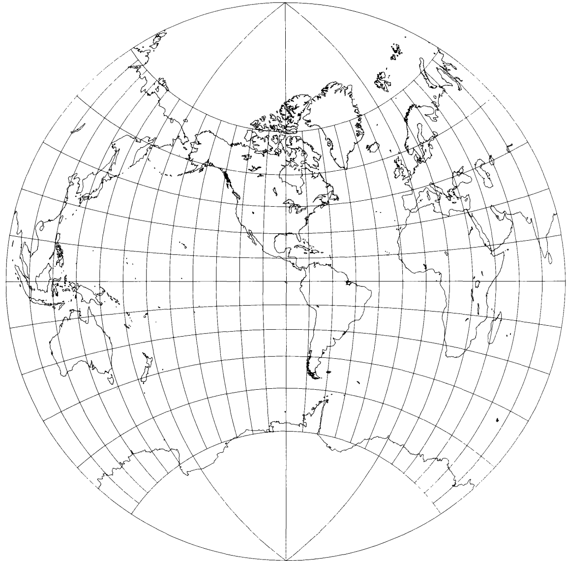
Figure 87.—Van der Grinten II projection, with shorelines, 15° graticule, central meridian 90° W.
