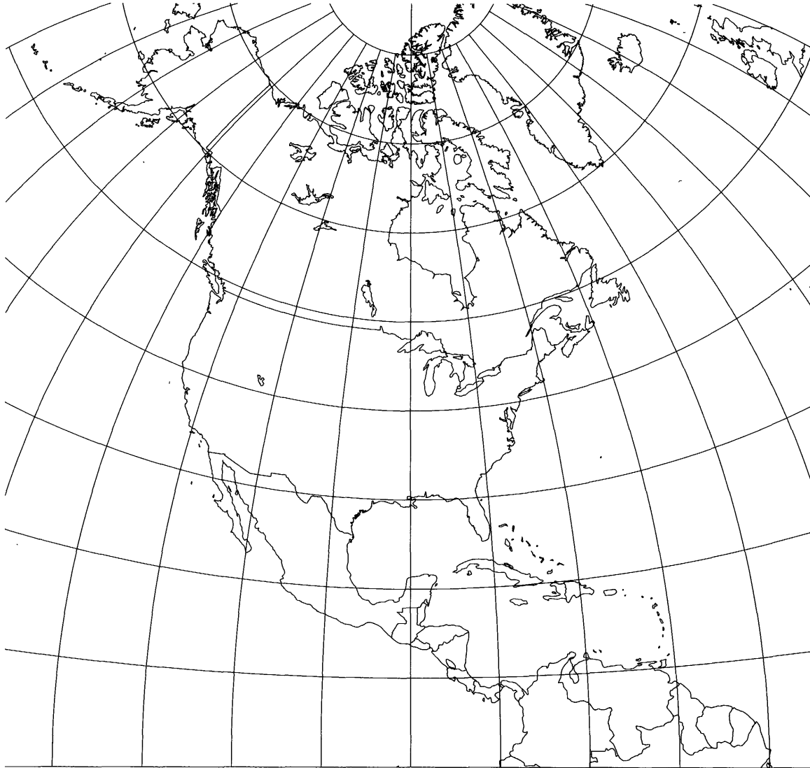
Figure 43B.—Polyconic projection, with shorelines, 10° graticule. Central meridian 90° W.
