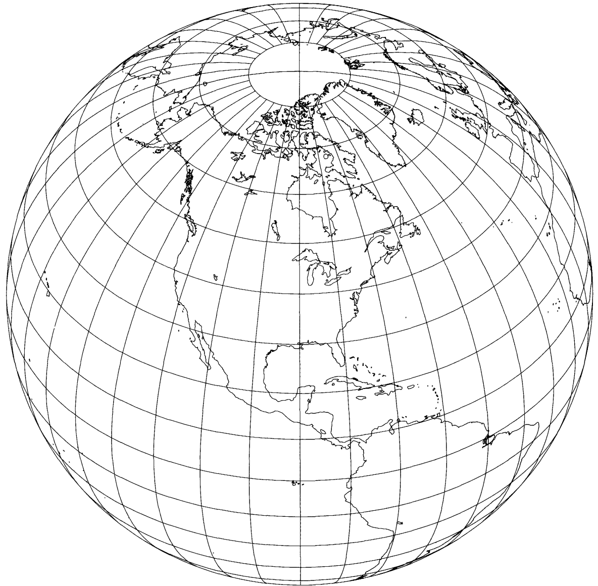
Figure 50D.—Oblique Orthographic projection, with shorelines, 10° graticule, central latitude 40° N. Central meridian 90° W.
