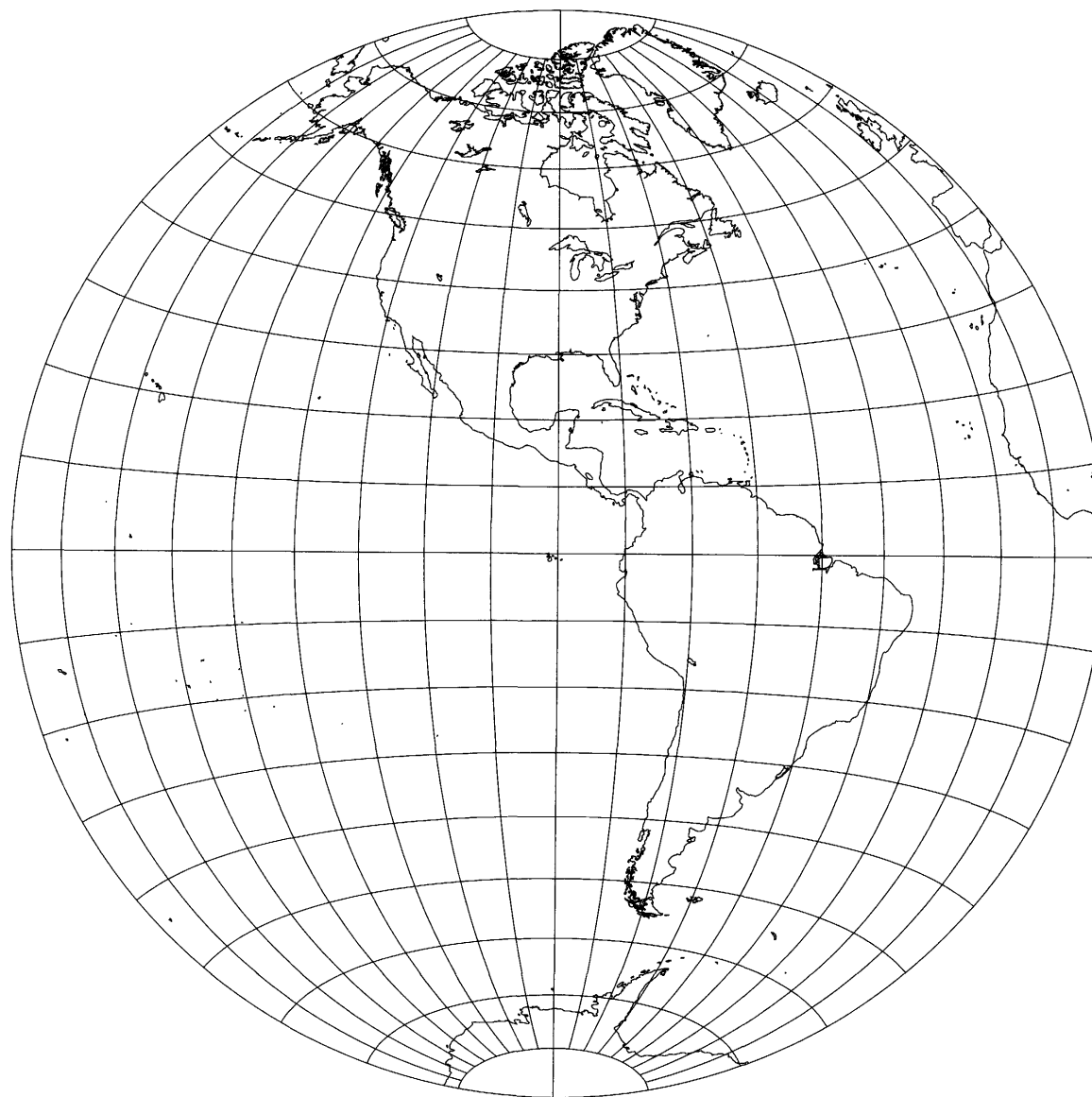
Figure 53C.—Equatorial Lambert Azimuthal Equal-Area projection, with shorelines, 105° graticule. Central meridian 90° W. Range 90°.
