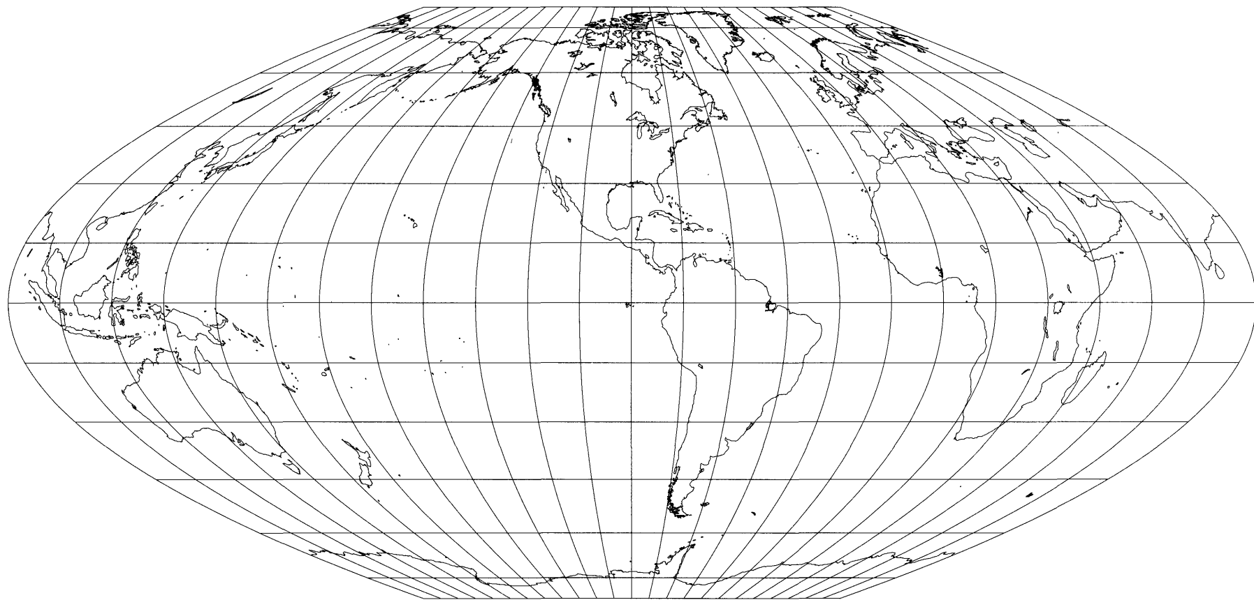
Figure 27B.—McBryde-Thomas Flat-Polar Parabolic projection, with shorelines, 15° graticule. Central meridian 90° W.
