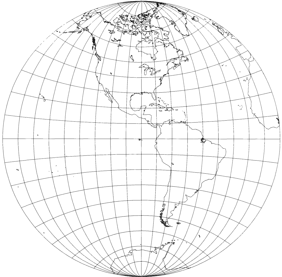
Figure 72.—Fournier Globular I projection, with shorelines, 10° graticule. Central meridian 90° W.
