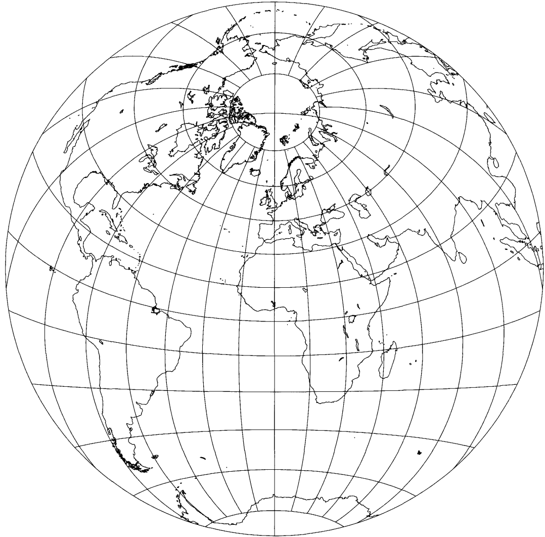
Figure 51D.—Clarke's Twilight projection, with shorelines, 15° graticule, central latitude 23.5° N. Central meridian 0°. Depth below surface 15,290 km. Range 108°.
