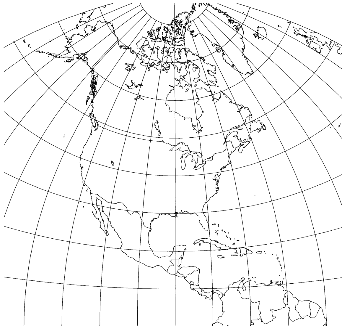
Figure 44.—Rectangular Polyconic projection, with shorelines, 10° graticule. Central meridian 90° W. Equator at true scale.
