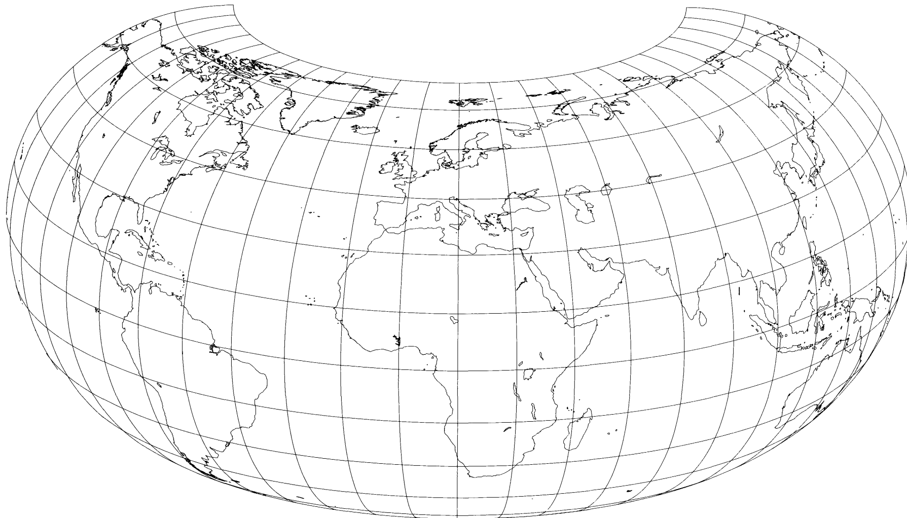
Figure 90.—Armadillo projection, with shorelines, 15° graticule, central meridian 15° E.
