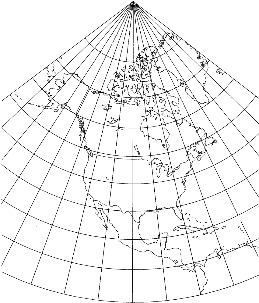
FIGURE 16.—Lambert Conformal Conic projection, with standard parallels 20^{\circ} and 60^{\circ} N. North America is illustrated here to show the change in spacing of the parallels. When used for maps of the conterminous United States or individual States, standard parallels are 33^{\circ} and 45^{\circ} N.
