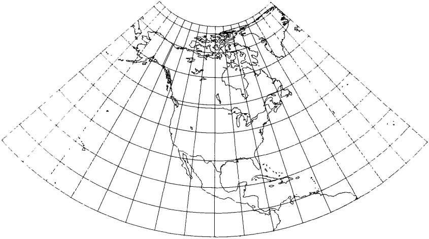
FIGURE 15.—Albers Equal-Area Conic projection, with standard parallels 20^{\circ} and 60^{\circ} N. This illustration includes all of North America to show the change in spacing of the parallels. When used for maps of the 48 conterminous States standard parallels are 29.5^{\circ} and 45.5^{\circ} N.
