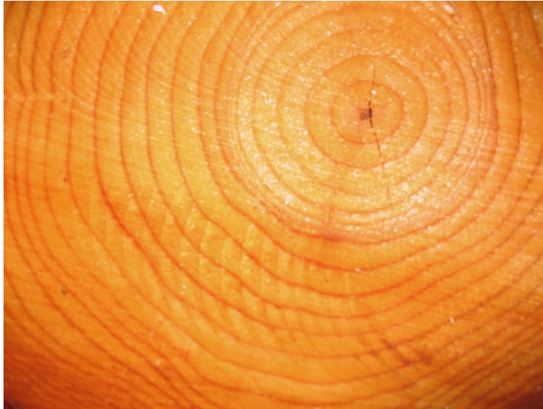
Figure 11.22: Cross-section showing growth rings. The thick, light-colored part of each ring represents rapid spring and summer growth. The thin, dark part of each ring represents slow autumn and winter growth. (3)
