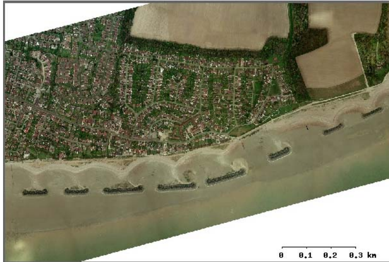
Figure 10.23: Breakwaters are visible in this satellite image, built parallel to the shoreline to protect areas from strong waves. (4)
