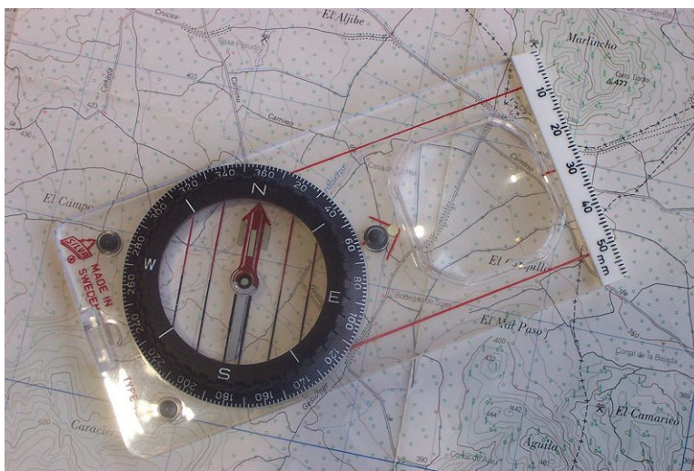
Figure 2.1: A compass is a device that is used to determine direction. The needle points to the Earth's magnetic north pole. (41)
