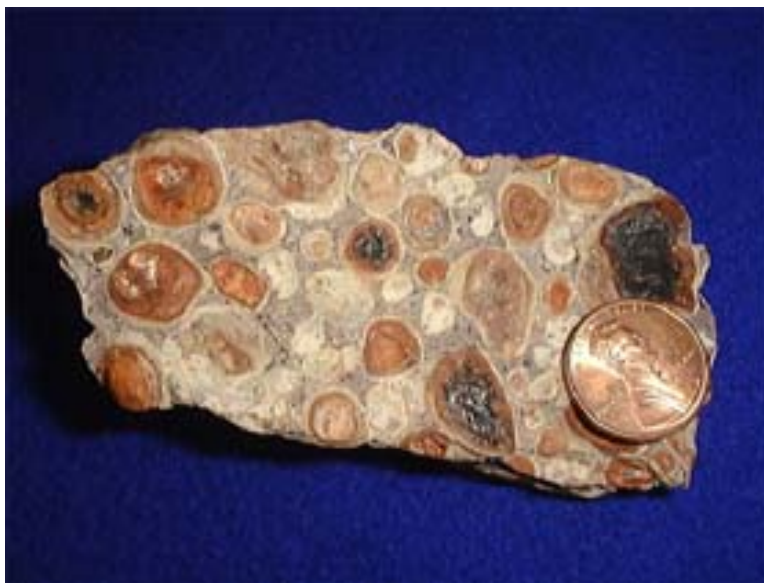
Figure 3.26: Aluminum is made from the minerals in rocks known as bauxite. (7)
