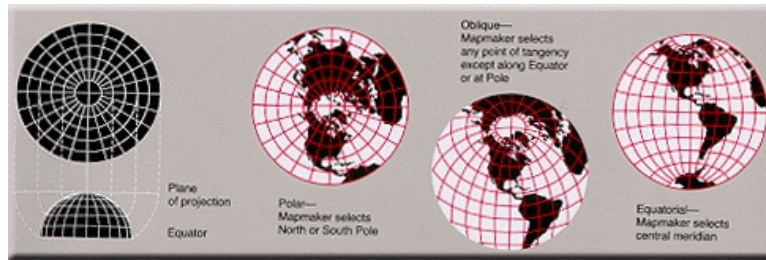
Figure 2.19: A gnomonic projection places a flat piece of paper on a point somewhere on Earth and projects an image from that point. (36)
