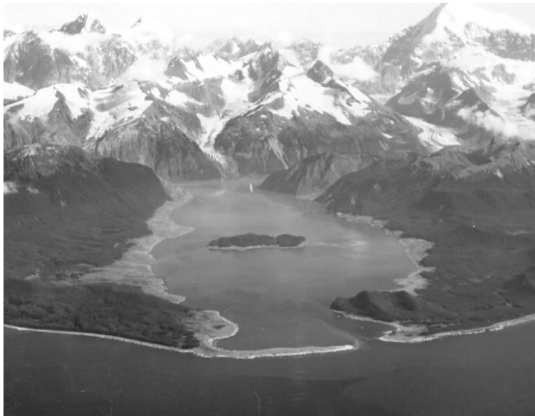
Figure 10.51: This photograph of Lituya Bay in Alaska shows (in light gray) the areas damaged by the tsunami produced by a landslide sent 30.6 million cubic meters of rock into the bay. (24)
