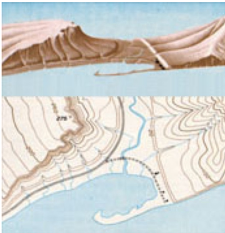
Figure 2.32: Illustrations of 3-dimensional ground configurations (top) and corresponding topographic map (bottom). Note the V-shaped markings on the topographic maps correspond to drainage channels. Also, the closely-spaced contour lines denote the rapid rising cliff face on the left side. (43)
