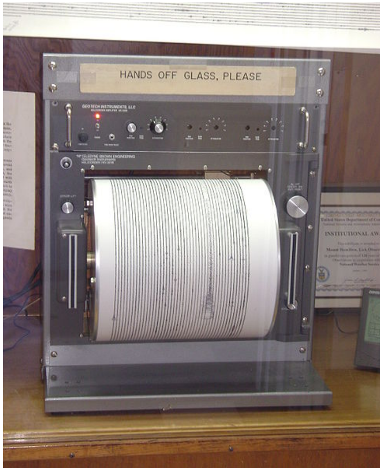
Figure 1.12: Seismographs are used to measure earthquakes and pinpoint their origins. (19)
