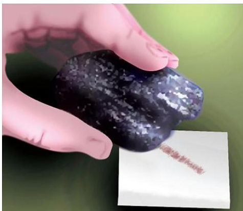
Figure 3.14: You rub a mineral across an unglazed porcelain plate to determine the streak. The hematite shown here has a red-brown streak. (23)
