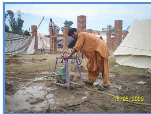
Figure 10. Hand driven donkey pump provided in Shah Mansoor Camp for Water Supply
