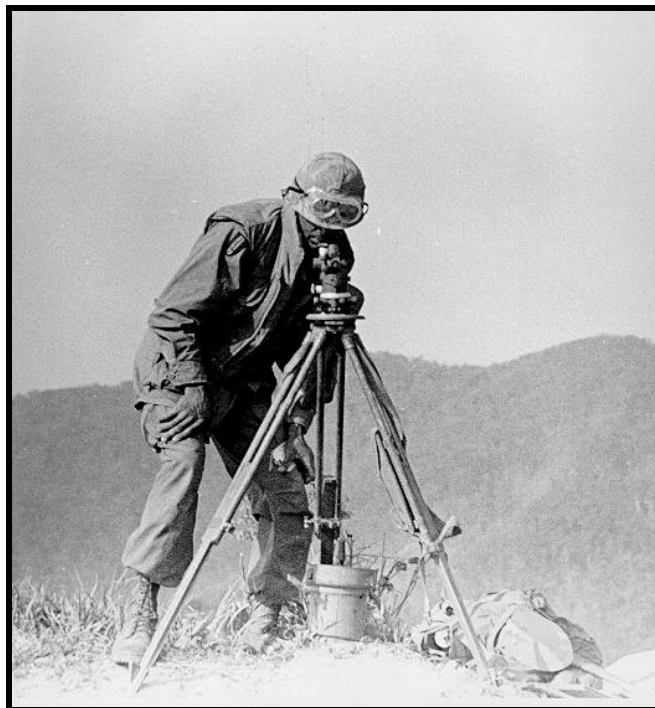
A Soldier of the 1-321 st Field Artillery Regiment uses an Aiming Circle to lay the M102 Howitzers in Vietnam
