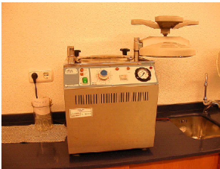
Figure 1.35: A worktop autoclave. Autoclaves commonly use steam heated to 121^{\circ}\text{C} ( 250^{\circ}\text{F} ), at 103\text{ kPa} ( 15\text{ psi} ) above atmospheric pressure. Solid surfaces are effectively sterilized when heated to this temperature. Liquids can also be sterilized by this process, though additional time is required to reach sterilizing temperature. (24)
