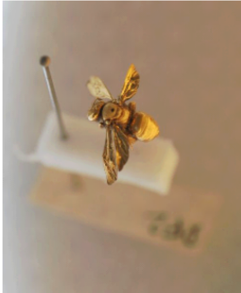
Figure 1.33: This insect has been coated in gold, as part of the preparation for viewing with an SEM. (12)
