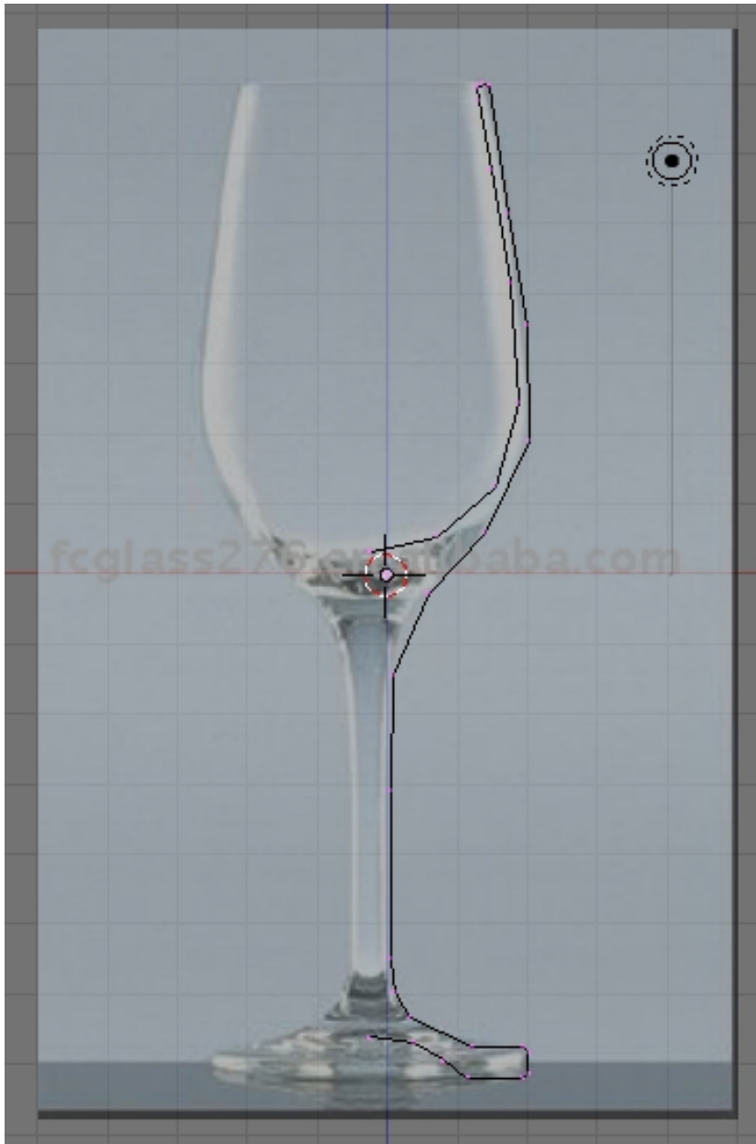
Figure 1387: Half outline of a wineglass with a background image as a guide
