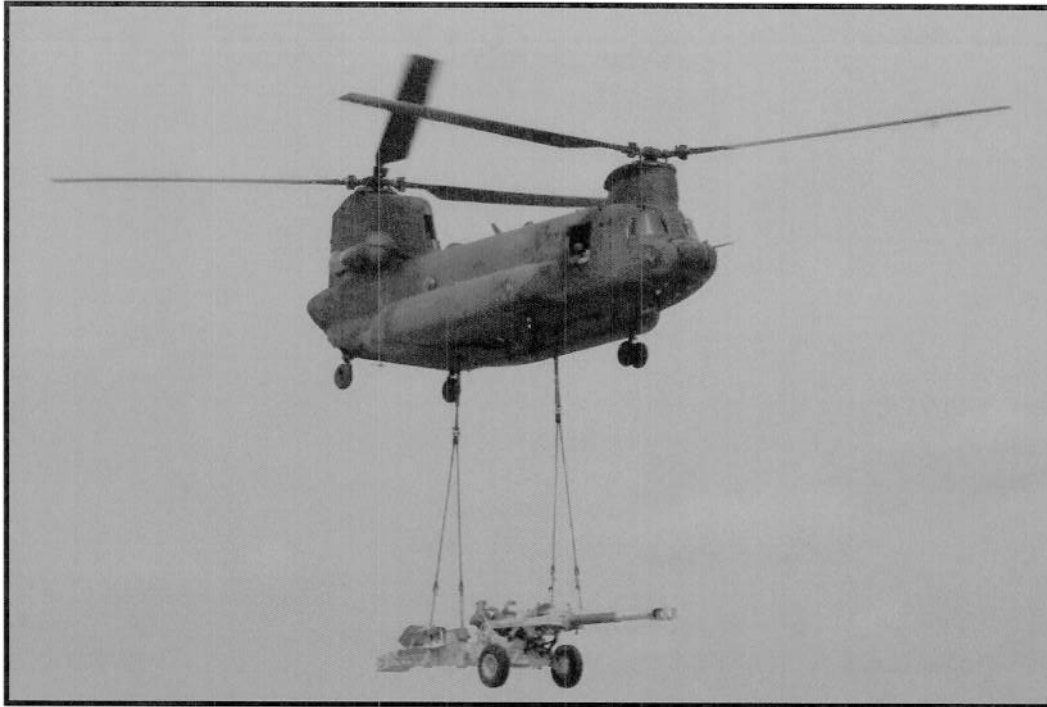
UH-77 Chinook Helicopter lifts a M198 Howitzer for an Air Assault Mission at Fort Bragg, NC.
