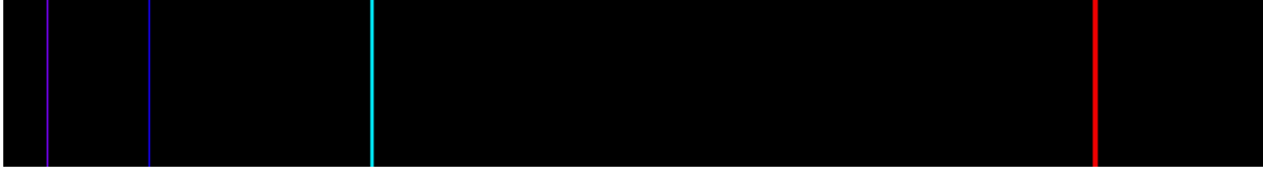
Abb. 21: Visible emission spectrum of atomic hydrogen, containing four lines of the BALMER SERIES 16 .
