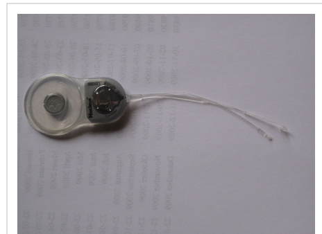
The internal part of a cochlear implant (model Cochlear Freedom 24 RE)
