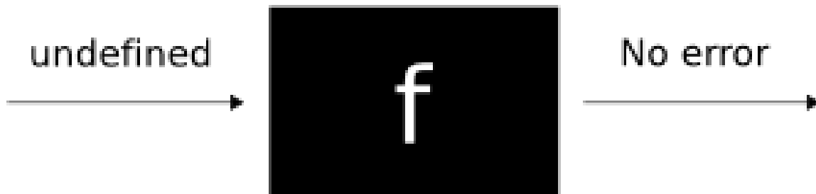
Figure 39: If f returns an error when passed undefined, it must be strict. Otherwise, it's lazy.
